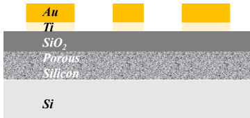
Fig. 2. Material stack used in the fabrication of CPW on PS.
