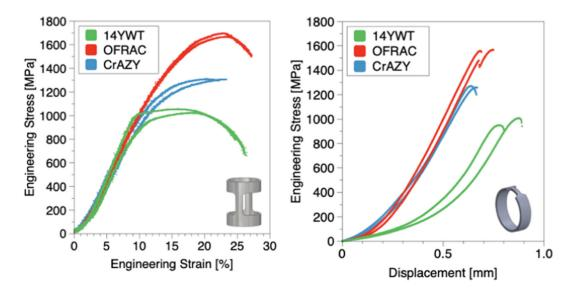
Fig. 11. Room temperature tensile response of axial (left) and ring-pull (right) specimens from each ODS tube. For axially loaded specimens, the engineering stress is plotted as a function of engineering strain, and for ring-pull specimens the stress is plotted as a function of crosshead displacement.
