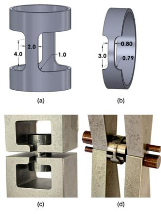
**Fig. 2.** Specimen types and dimensions used for (a) axial and (b) ring-pull tensile testing. The fixture used for axial tensile is shown in (c) and the fixture used for ring-pull tests is shown (d). Dimensions in (a) and (b) are given in millimeters.
