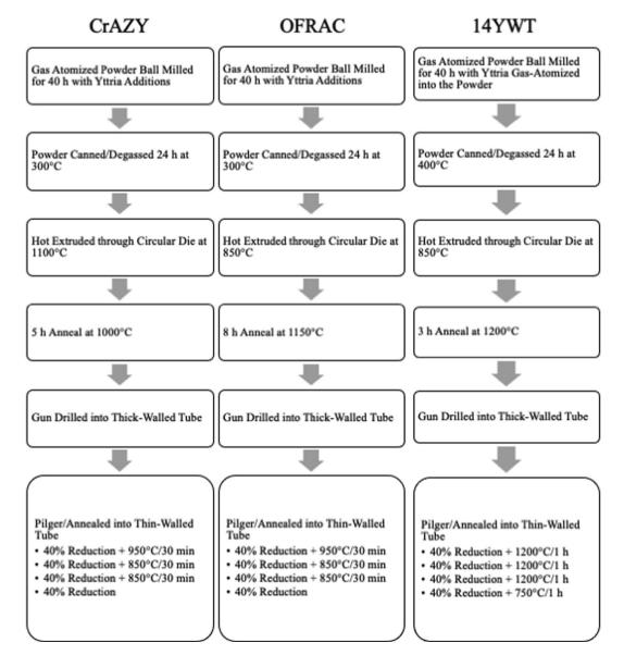
Fig. 1. Process diagrams for thin-walled ODS FeCr(Al) tubes produced via pilgering.
