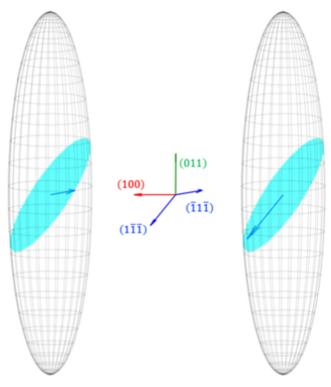
**Fig. 3.** Three-dimensional views of a spheroidal grain of aspect ratio 5:1 with major axis oriented parallel to [011] with resolved slip along  $(110)\begin{bmatrix} 1 & 1 \\ 1 & 1 \end{bmatrix}$  and  $(110)\begin{bmatrix} 1 & 1 \\ 1 & 1 \end{bmatrix}$ .
