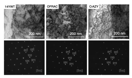
Fig. 6. Typical BF STEM images of dislocation networks in each ODS FeCr(Al) alloy tube. All micrographs are imaged along the (111)-zone axis, as confirmed by the accompanying indexed diffraction patterns.
