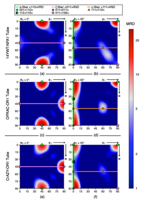
**Fig. 5.** ODF contour plots for each thin-walled tube computed from EBSD methods. All plots use Euler angle representation and highlight two characteristic slices at  $\phi_2 = 0^\circ$  and 45° where major rolling texture components for BCC materials are visible. All plots are normalized to the same color bar in units of multiples of random density.
