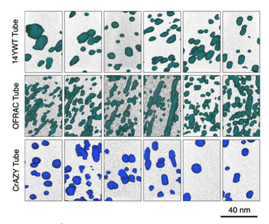
**Fig. 9.** APT volumes measuring  $40 \times 40 \times 65 \text{ nm}^3$  show the precipitate dispersions in each tube. Green isoconcentration surfaces highlight regions enriched in at least 1.5% (Y + Ti + O), and blue surfaces represent regions with 1.5% enrichment of (Y + Al + O). In each image, 0.1% of background Fe atoms are also presented as black dots. (For interpretation of the references to color in this figure legend, the reader is referred to the web version of this article.)
