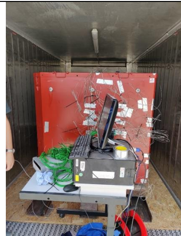
Figure 4 : Container with the external thermal sensors
