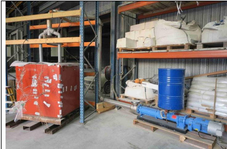
Figure 3 : Container (red) with the mortar injection apparatus
