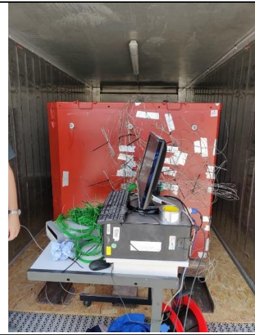
Figure 4 : Container with the external thermal sensors
