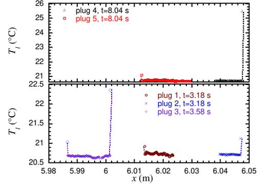
(a) Experimental distributions. The lines are put as an eye guide. The plug velocities are 0.018, 0.018, 0.018, 0.065 and 0.065 m/s for the plugs 1–5, respectively.  $T_{sat}(p_2)$  and  $T_{sat}(p_1)$  taken at the respective time moments are added as lower and upper bounds, respectively, for the interfacial values at the plug menisci.
