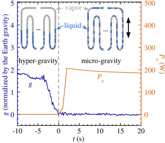
Figure 2: Evolution of the effective gravity acceleration  $g$  and the evaporator power for parabola 16. An illustrative distribution of the bubbles and the plugs is shown above for both accelerated and microgravity intervals.
