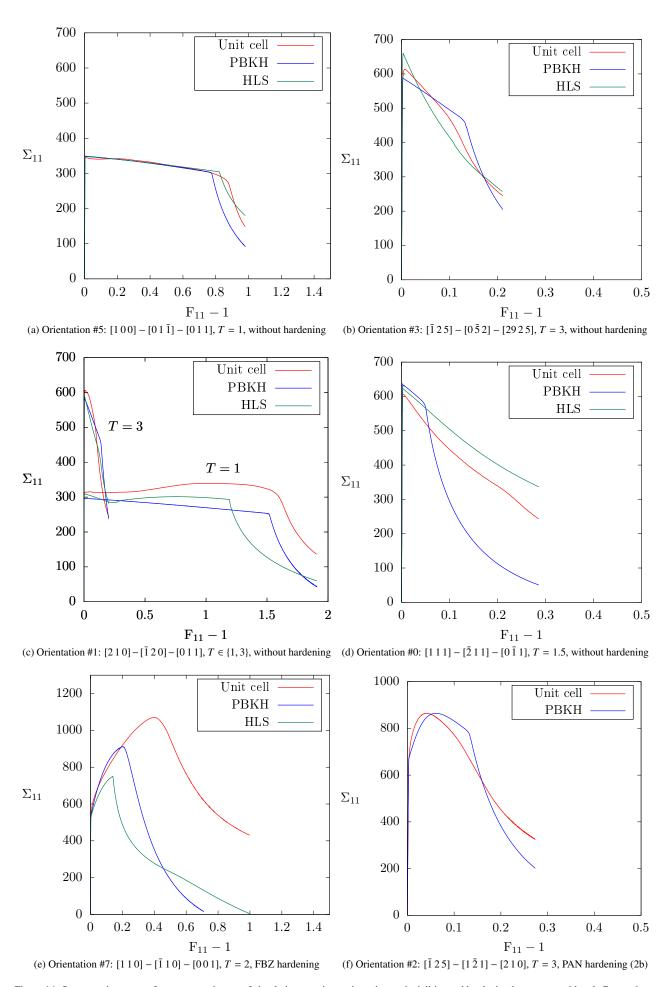
Figure 14: Stress-strain curves of a representative set of simulations: various orientations, triaxialities and hardening laws are considered. Comparisons are made between results of the unit-cell computation and predictions of the two homogenized models (PBKH and HLS).
