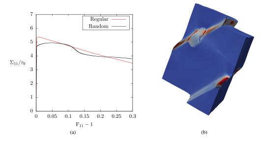
Figure 16: Finite strain porous ( $f_0 = 1\%$ ) single crystal ( $\phi_1 = 124.4^\circ$ ,  $\Phi = 34.2^\circ$ ,  $\phi_2 = 267.6^\circ$ ) unit-cell simulations under axisymmetric loading conditions (T = 1) without hardening, for regular (cubic void distribution) and random (with 8 voids): (a) stress-strain curves and (b) typical local deformation gradient field in the coalescence regime in the random case for  $F_{11} = 1.2$ .
