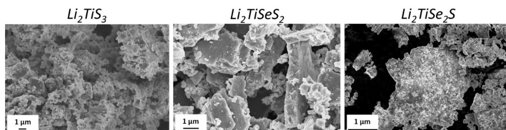
Figure 3. SEM images of \text{Li}_2\text{TiSe}_x\text{S}_{3-x} ( 0 \leq x \leq 2 ) materials.
