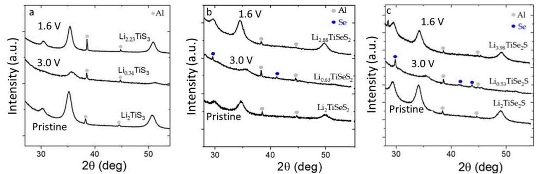
**Figure 7.** Ex situ X-ray diffractograms of (a)  $\text{Li}_2\text{TiS}_3$ , (b)  $\text{Li}_2\text{TiSe}_2$ , and (c)  $\text{Li}_2\text{TiSe}_2\text{S}$  electrodes at different states of charge: pristine, at the end of charge (3 V), and at the end of discharge (1.6 V).
