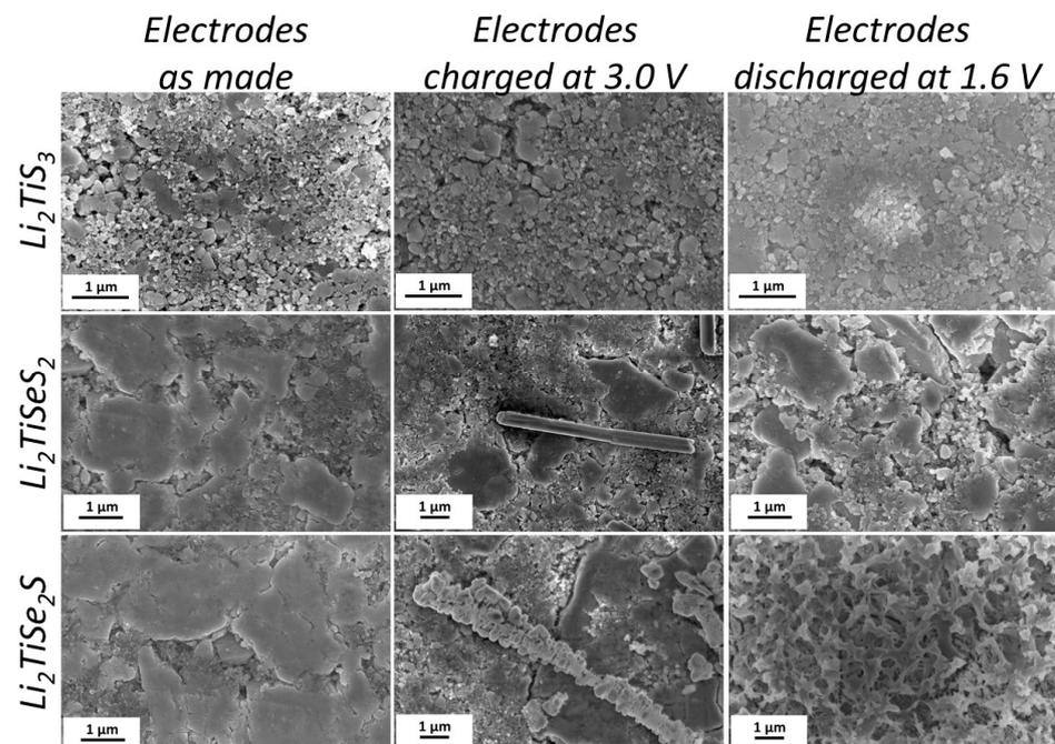
**Figure 8.** SEM images of  $\text{Li}_2\text{TiS}_3$ ,  $\text{Li}_2\text{TiSe}_2$ , and  $\text{Li}_2\text{TiSe}_2\text{S}$  electrodes at different states of charge: pristine, at the end of charge (3 V) and at the end of discharge (1.6 V).
