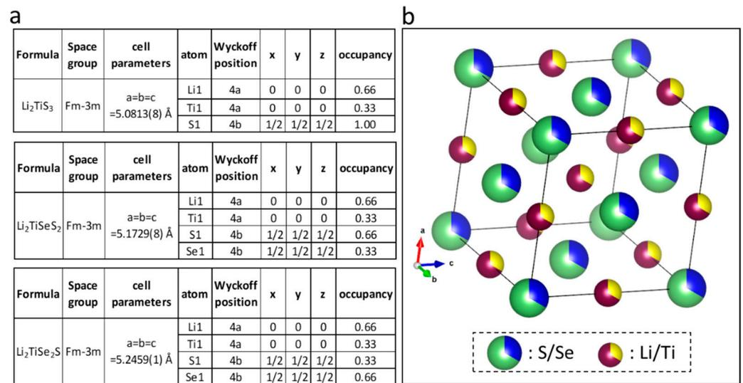
**Figure 2.** (a) Refined parameters of Li<sub>2</sub>TiSe<sub>x</sub>S<sub>3-x</sub> (0 ≤ x ≤ 2) materials and (b) Li<sub>2</sub>TiSeS<sub>2</sub> structure.
