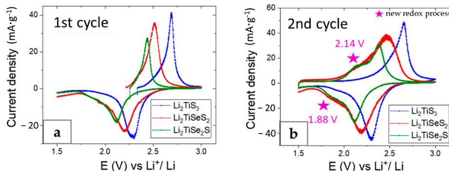
**Figure 5.** Redox potentials comparison of  $\text{Li}_2\text{TiS}_3$ ,  $\text{Li}_2\text{TiSeS}_2$ , and  $\text{Li}_2\text{TiSe}_2\text{S}$  electrodes at the first ( $5 \mu\text{V}\cdot\text{s}^{-1}$ ) (a), and second ( $10 \mu\text{V}\cdot\text{s}^{-1}$ ) (b) cycles between 3 and 1.5 V vs.  $\text{Li}^+/\text{Li}$ .
