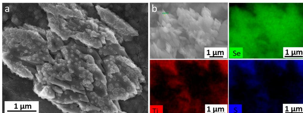
**Figure 9.** (a) SEM images and (b) EDX images of  $\text{Li}_2\text{TiSe}_2\text{S}$  electrodes charged to 3 V and kept for 24 h.
