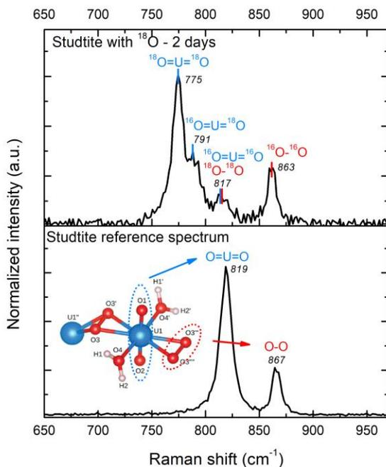
Figure 2 : Raman spectra of studtite formed at the surface of the MIMAS MOX sample after two leaching days in <sup>18</sup>O-enriched water (top) and formed in water of natural isotopic composition (bottom) with bands assignment and ball-and-stick representation<sup>31</sup>.
