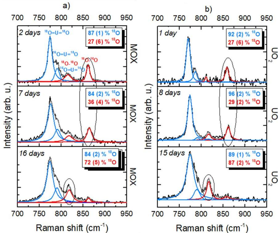
Figure 4 : Evolution through time of the studtite spectra for: a) a MOX sample compared to b) a UO<sub>2</sub> sample. The mean isotopic enrichment of the uranyl (blue) and peroxide (red) bonds are indicated on each graph with the standard deviation in parentheses.
