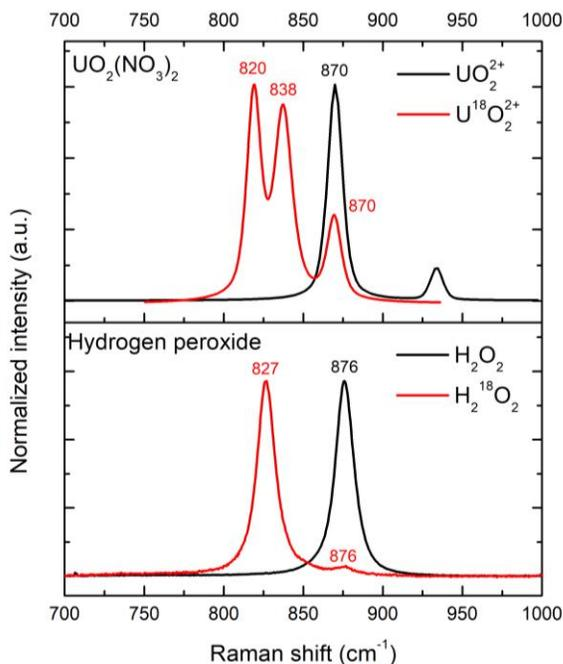
Figure 3 : Raman spectra of: top  $\text{UO}_2^{2+}$ <sup>32</sup> (the peak at  $933\text{ cm}^{-1}$  is due to the  $\text{ClO}_4^-$  internal standard) and  $\text{U}^{18}\text{O}_2^{2+}$ <sup>33</sup>; bottom:  $\text{H}_2\text{O}_2$  and  $\text{H}_2^{18}\text{O}_2$  (enriched in 97% in  $^{18}\text{O}$ ) at 1M concentration analyzed during this study.
