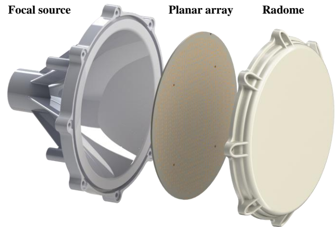
Fig. 1. Exploded view of the complete transmitarray antenna.
