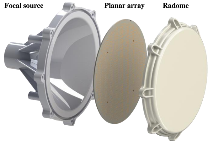
Fig. 1. Exploded view of the complete transmitarray antenna.
