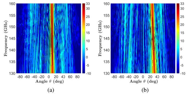
Fig. 12. Measured gain pattern (in dBi) as a function of frequency and elevation angle in the E-plane for the two transmitarrays steering the antenna beam at: (a)  $\theta_0 = 10^\circ$  (Lens 2) and (b)  $\theta_0 = 30^\circ$  (Lens 3).
