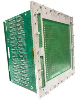
Fig. 3. Photograph of the assembled antenna prototype.
