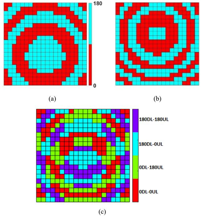
Fig. 5. Phase distribution layout for broadside radiation: (a) downlink, (b) uplink and (c) final combined layout.
