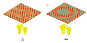
Fig. 4. Dual-band transmitarray showing two independent phase distribution, (a) for the uplink and (b) for the downlink.
