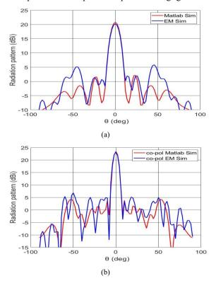
Fig. 7. Simulated radiation pattern for both bands (a) downlink and (b) uplink
