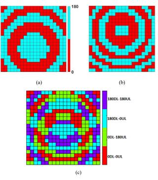
Fig. 5. Phase distribution layout for broadside radiation: (a) downlink, (b) uplink and (c) final combined layout.
