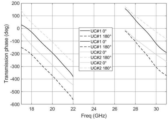
Fig. 2. Computed transmission phase of UC#1 and UC#2.
