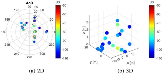
Fig. 4. Omnidirectional PADP extracted from VCA measurements.
