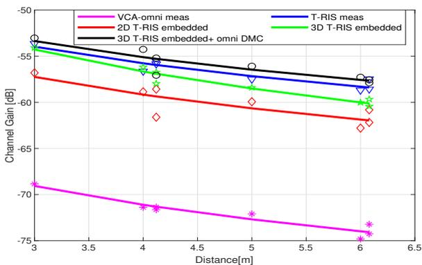
Fig. 10. Channel gain comparison: measurements vs models.
