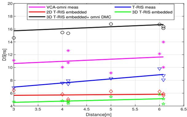
Fig. 11. Delay Spreads comparison: measurements vs models.
