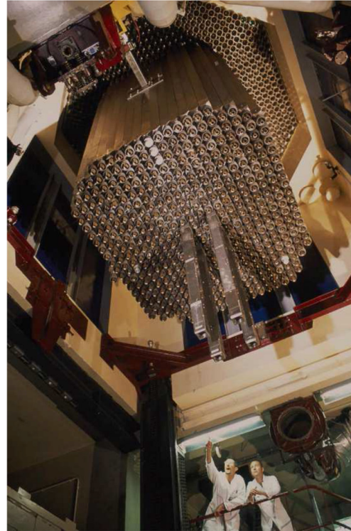
Fig. 12. The MUSE-4 Program: radical critical configuration (left), and actual MASURCA configuration (right: one can observe the GENEPI accelerator channel entering the core on the upper-left part).
