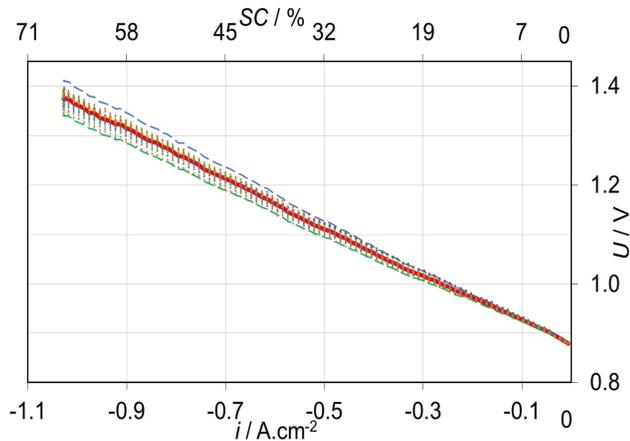
Figure 5: Cell voltage typical scattering recorded for a stack operated in SOEC providing 90/10 vol.% H<sub>2</sub>O/H<sub>2</sub> mix to the fuel electrode at 700°C. Cells voltage data are plotted with circle marks, the associated median cell voltage is plotted as a red continuous line, two dotted lines derived from median voltage curve highlight cell voltage scattering remains within  $\pm 7\%$ .
