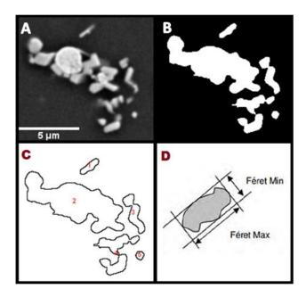
Figure 6 – Example of the image treatment applied to the SEM images to identify the structural units of PGM particles: a) Raw image from SEM. b) The same image after treatment with the Fiji program. c) Contours of the SUs after treatment. d) An example of the Féret form.
