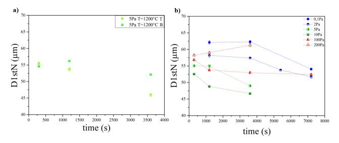
Figure 8- a) Average distance distribution of the particles first neighbor for the 5 Pa samples as a function of time for the top (T) and the bottom (B) of the crucible. b) Average distance distribution of the particles first neighbor for all the studied stresses as a function of time.
