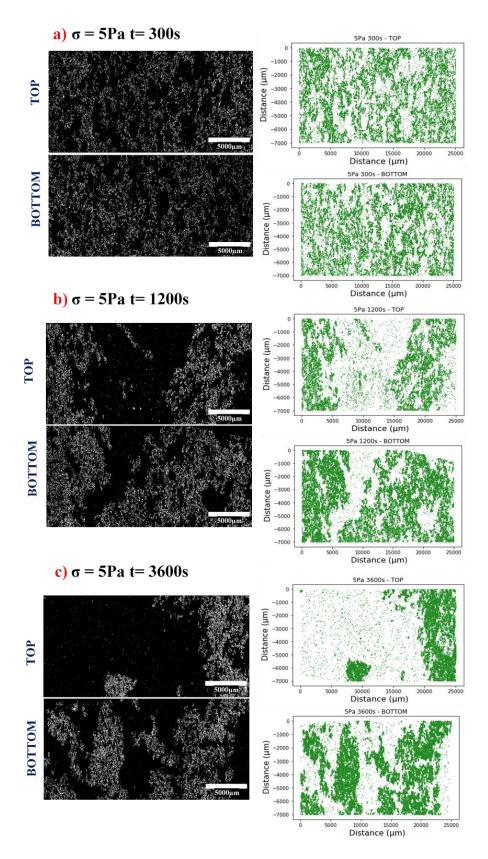
Figure 7 – Top and bottom SEM images (left column) of the sample subject to 5 Pa stress for 3 different durations, binarized via image treatment, along with their corresponding Cartesian representations (right column) of the PGM structural units positioning. Durations of the tests: a) 300 s b) 1200 s, and c) 3600 s.
