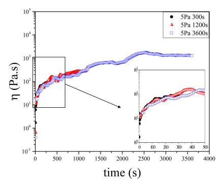
Figure 5 – Evolution of viscosity in time at the imposed stress of 5 Pa for three different samples tested during 300 s, 1200 s and 3600 s. The zoom focuses on the overlap of the three curves, indicating the reproducibility of the experiments.
