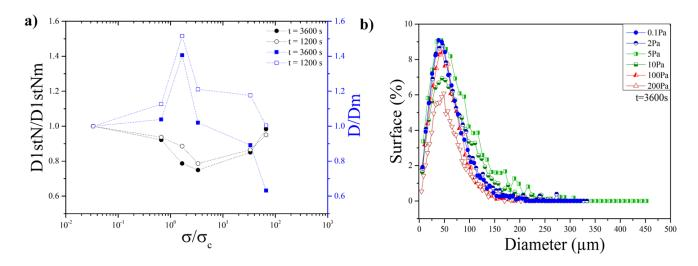
Figure 10 - a) Normalized D1stN and normalized Féret diameter (D) as a function of the normalized shear stress for experimental durations t = 3600 s and t = 1200 s. b) Surface percentage as a function of the cluster diameters for all the 3600s-samples studied.
