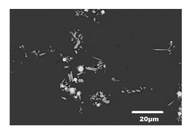
Figure 1 – Scanning Electron Microscopy (SEM) micrographs taken using back-scattered electrons (BSE) mode under 1000X magnification for the technological nuclear glass containing 3 wt% PGM particles after vitrification.
