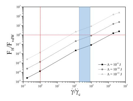
Figure 12 – The ratio between the hydrodynamic forces (F<sub>H</sub>) and the van der Walls potential (F<sub>vdW</sub>) as a function of  $\dot{\gamma}/\dot{\gamma}_c$ , for three different Hamaker constants.  $\dot{\gamma}_c$  is the critical shear rate when the viscosity abruptly decreases.
