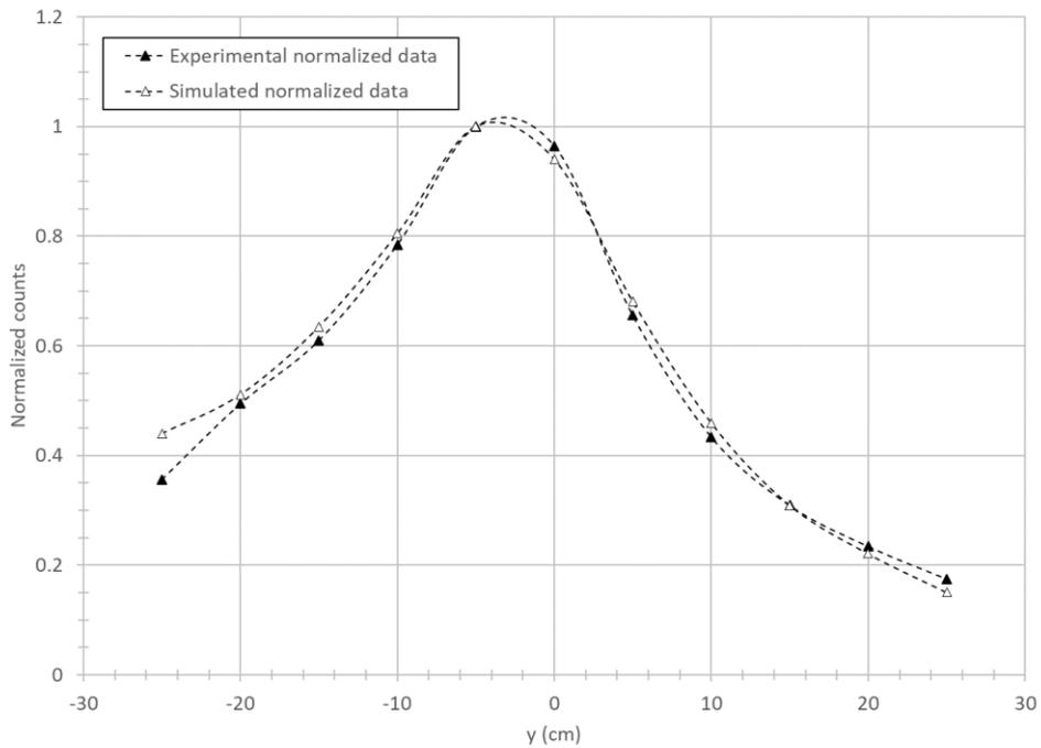
Figure 16. Comparison of the horizontal scanning of the drum obtained using the MCNP6 model with the experimental data acquired at the SAPHIR platform.
