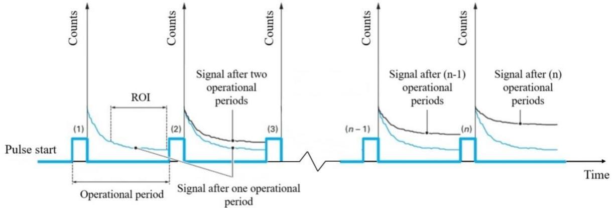
Fig. 3. Schematic chronogram of the interpulse counting mode of delayed neutrons from photofission.
