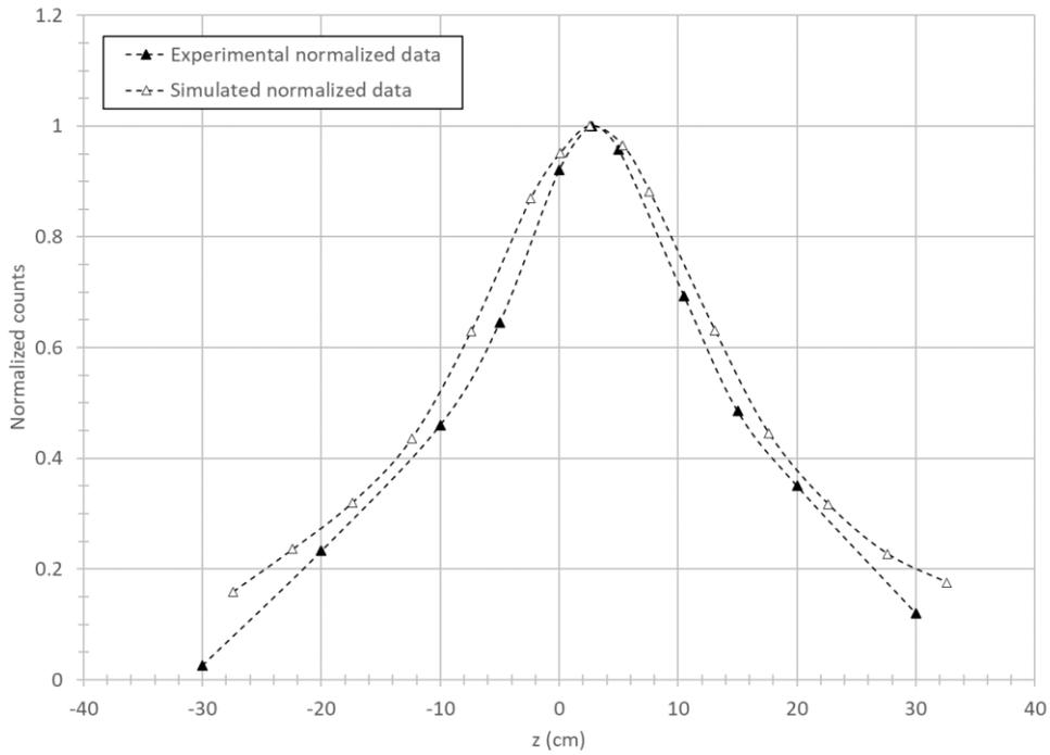
Figure 15. Comparison of the vertical scanning of the drum obtained using the MCNP6 model with the experimental data acquired at the SAPHIR platform.
