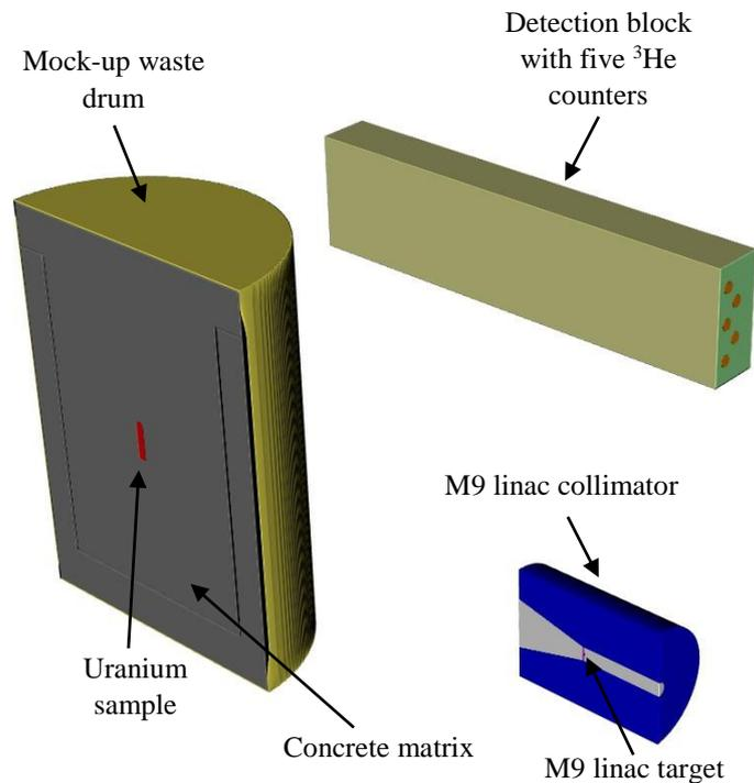
Fig. 17. Virtual concrete filled mock-up drum case.
