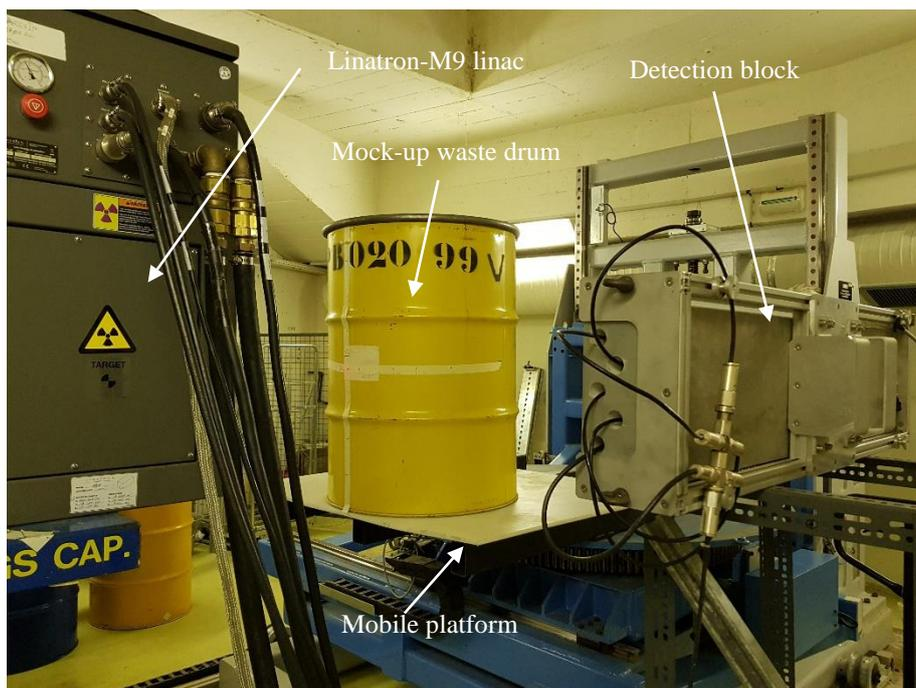
Fig. 2. Overview of the experimental setup at the SAPHIR platform (CEA Paris-Saclay).
