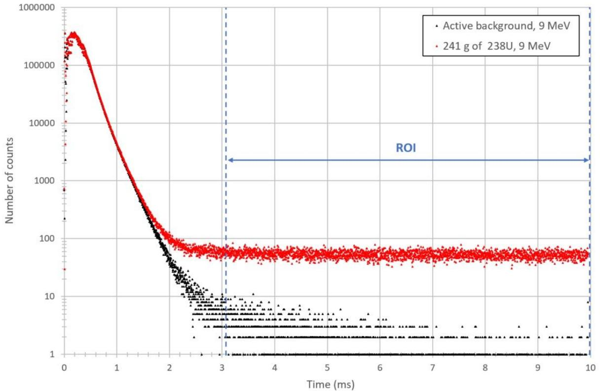
Fig. 6. Measured response from depleted uranium sample and active background at 9 MeV integrated for the 60000 irradiation cycles.
