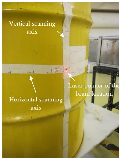
Fig. 11. Mock-up drum positioning geometry.
