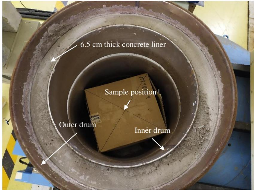
Fig. 4. Mock-up drum with a concrete liner.
