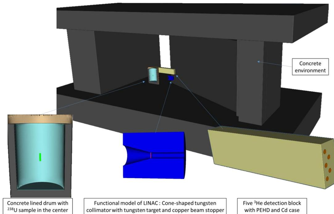
Fig. 5. 3D view of the MCNP6 simulation model.
