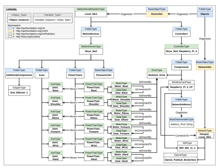
Fig. 3. OPC UA Information Model after integrating Niryo Ned and PubSub UDP UADP protocol into the LocalSEA testbed
