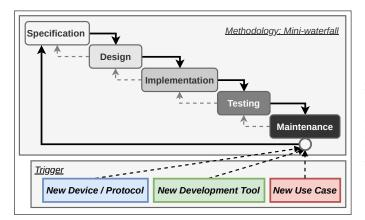
Fig. 1. Testbed development methodology: Mini-waterfall with triggers
