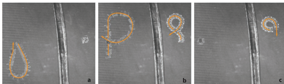
Figure 5. Two MagMites independently operating on the same surface, with motion paths illustrated. MagMites are separated by a polymer wall. Adapted with permission. [101] Copyright 2011, SAGE.
