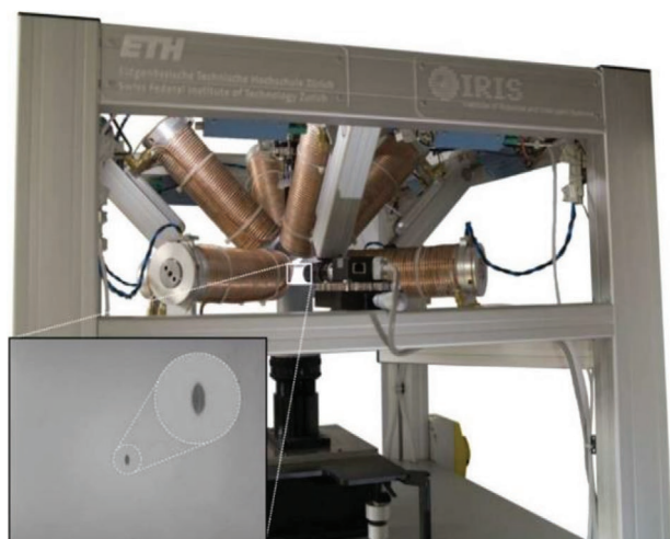
Figure 8. Experimental apparatus of the Octomag system, showing eight electromagnetic coils surrounding a workspace. Inset shows an optical image of an oval-shaped magnetic microrobot in the workspace. Adapted with permission. [85] Copyright 2009, IEEE.
