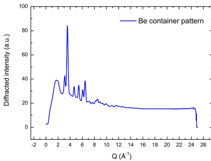
Fig. 5: Absorption from the Be container. Abcissa is referred as momentum transfer (in  $\text{\AA}^{-1}$ ).
