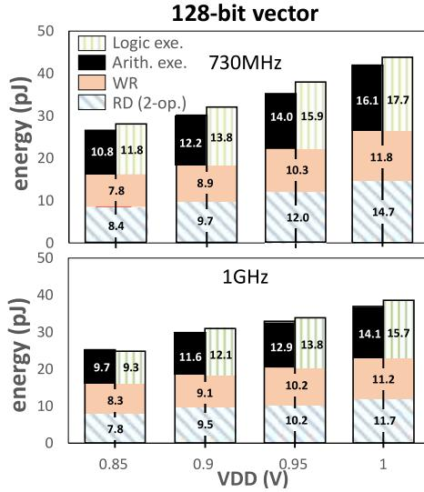
Fig. 6. Measured logic and arithmetic instruction energy versus VDD.
