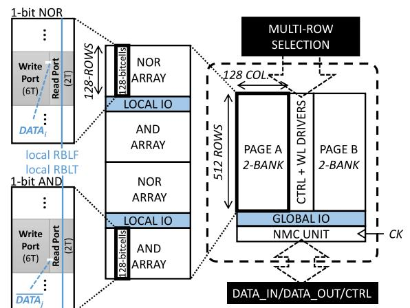
Fig. 3. Proposed C-SRAM architecture based on two adjacent memory pages.
