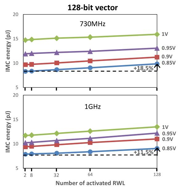
Fig. 7. Measured IMC energy versus number of activated RWL.
