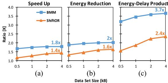
Fig. 10. Simulated (a) speed-up, (b) energy reduction, and (c) EDP ratio of 128-b C-SRAM versus 128-b SIMD processor (baseline).
