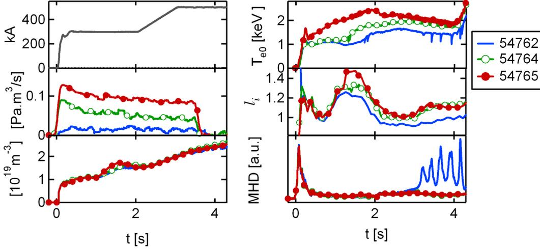
**Figure 1.** Example of 3 consecutive pulses (54762, 54764, 54765) with increasing Nitrogen seeding rate. Left column: plasma current (top), Nitrogen injection rate (middle) and volume averaged plasma density (bottom). Right column: central electron temperature, internal inductance and MHD level.
