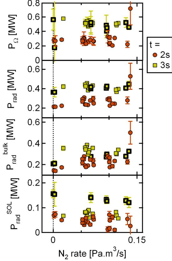
**Figure 5.** From top to bottom: ohmic power, total, bulk and SOL radiated powers at  $t = 2\text{s}$  and  $t = 3\text{s}$  as a function of the Nitrogen injection rate. Bold symbols correspond to the series with a higher density at  $t = 3\text{s}$ .
