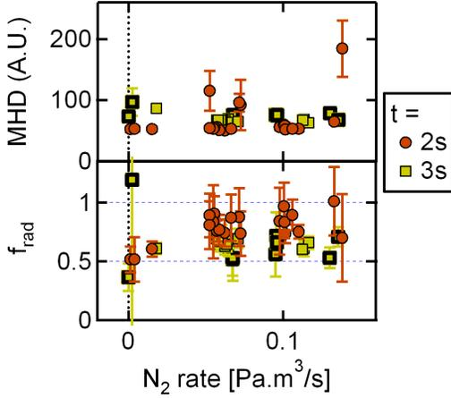
**Figure 6.** MHD activity recorded by Mirnov coils (top) and radiative fraction  $P^{bulk}/P_{\Omega}$  (bottom), at  $t = 2s$  and  $t = 3s$  as a function of the Nitrogen injection rate. Bold symbols correspond to the series with a higher density at  $t = 3s$ .
