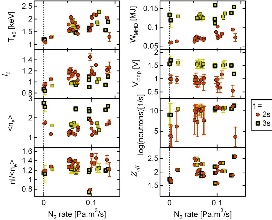
**Figure 4.** Central electron temperature, internal inductance, volume averaged density, density peaking, energy content, loop voltage, neutron rate and resistive  $Z_{eff}$ , at  $t = 2s$  and  $t = 3s$  as a function of the Nitrogen injection rate. Bold symbols correspond to the series with a higher density at  $t = 3s$ .
