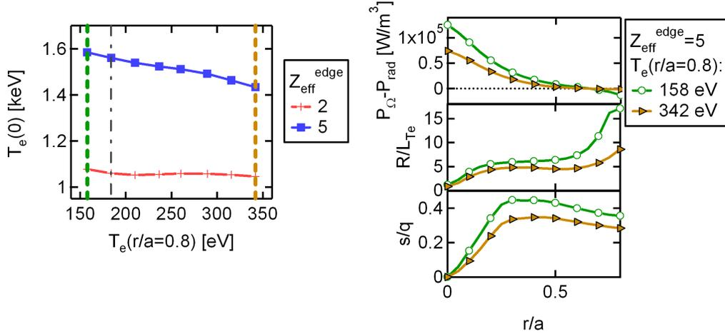
**Figure 24.** Left: Core electron temperature with ( $Z_{eff}^{edge} = 5$ ) and without ( $Z_{eff}^{edge} = 2$ ) Nitrogen injection, as a function of the temperature prescribed at  $r/a = 0.8$ . Right: profiles of the net heat source, normalized temperature gradient and  $s/q$  at  $Z_{eff}^{edge} = 5$  for the lowest and highest temperature at the boundary. The thin vertical line indicates the default value used in this study ( $c_W = 10^{-4}$ , no sawtooth model).
