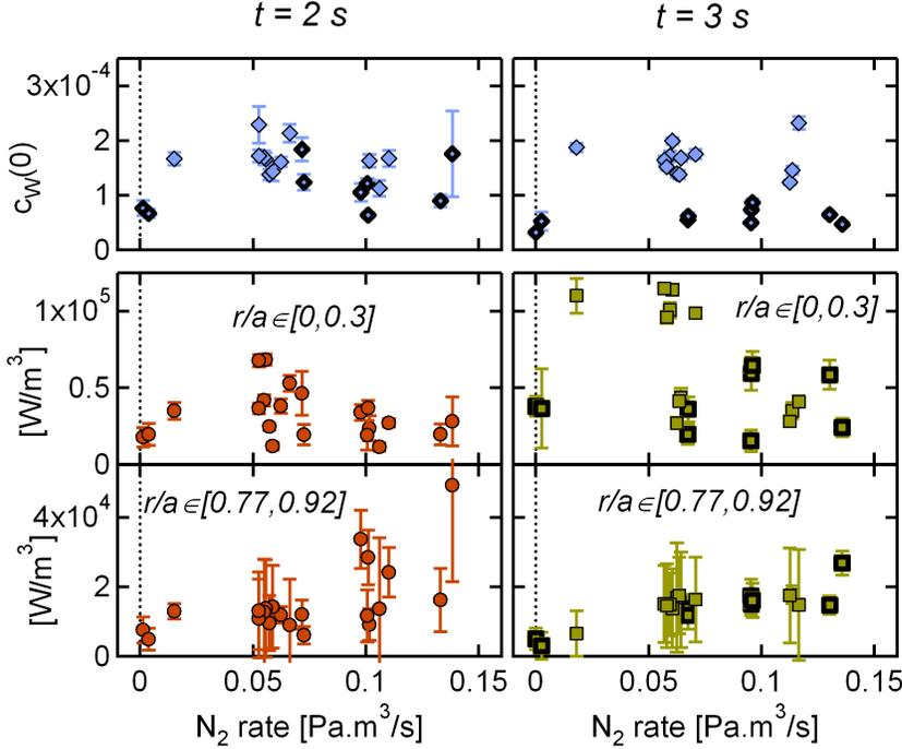
**Figure 11.** Bolometry inversion: from top to bottom, Tungsten concentration deduced from core radiation, radiative power emission in the core region and in the edge region, as a function of the Nitrogen injection rate at  $t = 2\text{ s}$  (left column) and  $t = 3\text{ s}$  (right column). Bold symbols correspond to the series with a higher density at  $t = 3\text{ s}$ .
