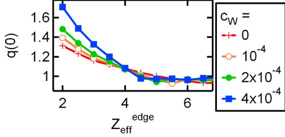
**Figure 17.** Central safety factor value at  $t = 2s$  as a function the edge  $Z_{eff}$ , for different levels of Tungsten concentration.
