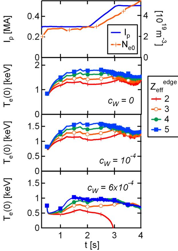
**Figure 19.** RAPTOR simulations: time evolution of the prescribed plasma current and central electron density (top), and of the predicted central electron temperature without Tungsten, and with a relative fraction of  $10^{-4}$  and  $6 \times 10^{-4}$ , for different values of the edge  $Z_{eff}$  with  $Z_{eff} = 2 + Z_{eff}^{edge} (r/a)^2$ .
