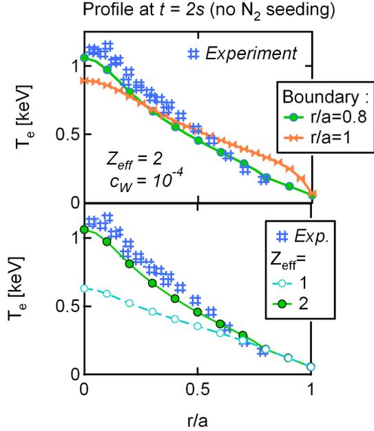
**Figure 13.** Top : Experimental and simulated electron temperature profiles at  $t = 2s$  for a boundary condition at  $r/a = 1$  and  $r/a = 0.8$  for a non-seeded case (flat  $Z_{eff} = 2$ ,  $c_W = 10^{-4}$ ). Below: effect of background light impurity content.
