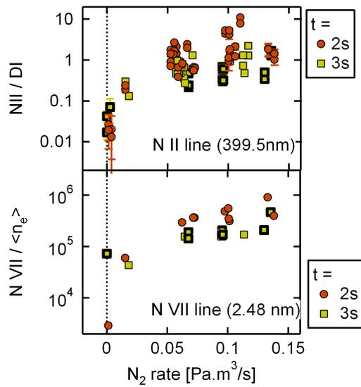
**Figure 9.** Top: Emission of the Nitrogen II line at 399.5nm normalized to the Deuterium I line at 434.1nm measured at the inner and outer strike points, at  $t = 2s$  and  $t = 3s$  as a function of the Nitrogen injection rate. Bottom: emission of the Nitrogen VII line at  $t = 2s$  and  $t = 3s$  as a function of the Nitrogen injection rate. Bold symbols correspond to the series with a higher density at  $t = 3s$ .
