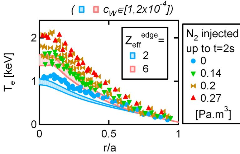
**Figure 15.** Electron temperature profile from the reference pulse without Nitrogen seeding (55797) and the following pulses with increasing levels of Nitrogen injection, compared to RAPTOR simulations with  $Z_{eff}^{edge} = 2$  and  $Z_{eff}^{edge} = 6$ , at  $t = 2$ s, for Tungsten concentration between  $10^{-4}$  and  $2 \times 10^{-4}$ .
