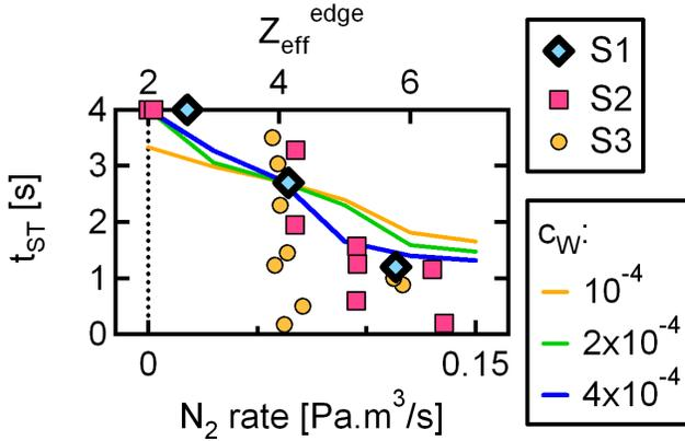
**Figure 18.** Time of appearance of sawtooth regime as a function of the N2 injection rate for experimental data (S1, S2 and S3 are three of the four series of pulses included in the database), and of  $Z_{eff}^{edge}$  for simulation data with different levels of Tungsten concentration.
