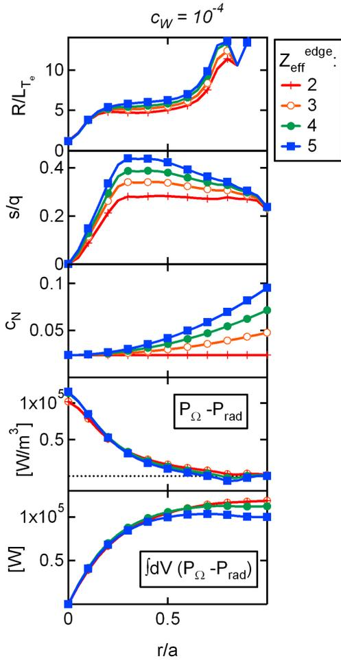
**Figure 20.** RAPTOR simulations: normalized electron temperature gradient  $R/L_{T_e}$ ,  $s/q$  parameter, Nitrogen concentration  $c_N = n_N/n_e$ , net power density and net cumulative heat source profiles at  $t = 2$ s, for a Tungsten concentration  $c_W = 10^{-4}$ .
