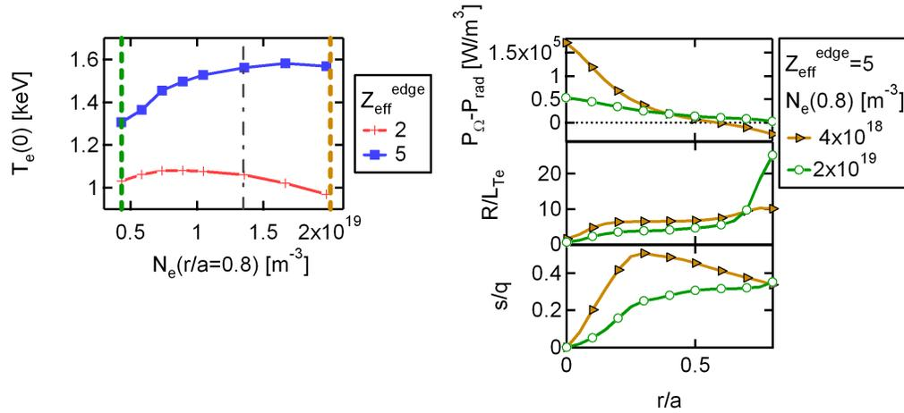
**Figure 25.** Left: Core electron temperature with ( $Z_{eff}^{edge} = 5$ ) and without ( $Z_{eff}^{edge} = 2$ ) Nitrogen injection, as a function of the density prescribed at  $r/a = 0.8$ . Right: profiles of the net heat source, normalized temperature gradient and  $s/q$  at  $Z_{eff}^{edge} = 5$  for the lowest and highest density at the boundary. The thin vertical line indicates the default value used in this study ( $c_W = 10^{-4}$ , no sawtooth model).
