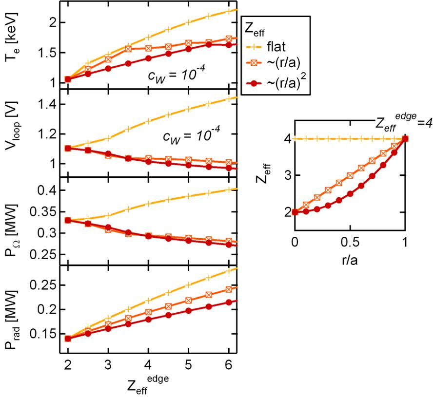
**Figure 14.** RAPTOR simulations, from top to bottom: central electron temperature, loop voltage, ohmic power and radiated power at  $t = 2s$  as a function of the edge  $Z_{eff}$  for a flat profile, and for profiles varying as  $(r/a)$  and  $(r/a)^2$  (case with  $c_W = 10^{-4}$ ,  $Z_{eff}(0) = 2$ ). An example of the corresponding  $Z_{eff}$  profiles is shown in the right plot for  $Z_{eff}^{edge} = 4$ .
