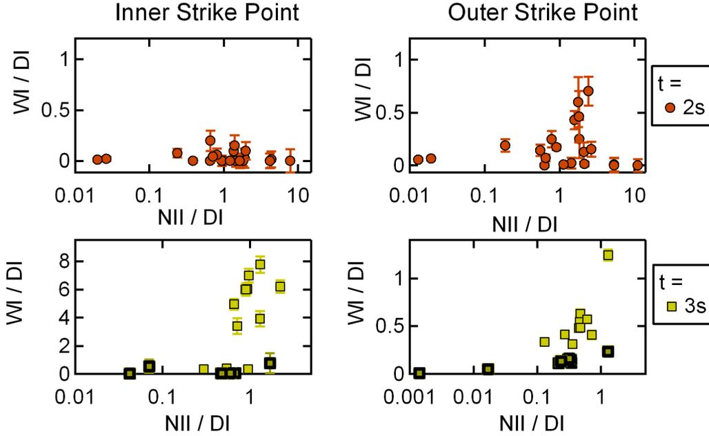
**Figure 10.** Emission of the Tungsten I line at 400.9nm normalized to the  $D_\gamma$  (434.1nm) brightness on the inner (left plots) and outer (right plots) strike points, as a function of the normalized Nitrogen II line at 399.5nm, at  $t = 2s$  (top) and  $t = 3s$  (bottom plots). Bold symbols correspond to the series with a higher density at  $t = 3s$ .
