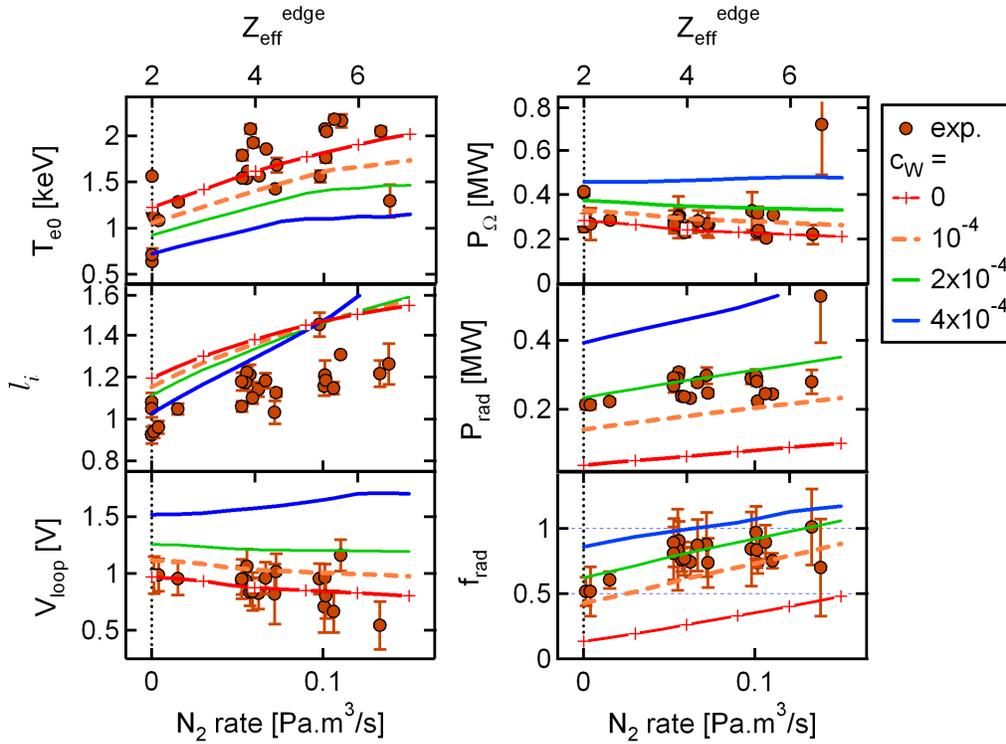
**Figure 16.** Core electron temperature, internal inductance, loop voltage, ohmic power, radiated power and radiated power fraction at  $t = 2$ s as a function of  $N_2$  injection rate for experimental data, and of  $Z_{eff}^{edge}$  for simulation data, with different levels of Tungsten concentration.
