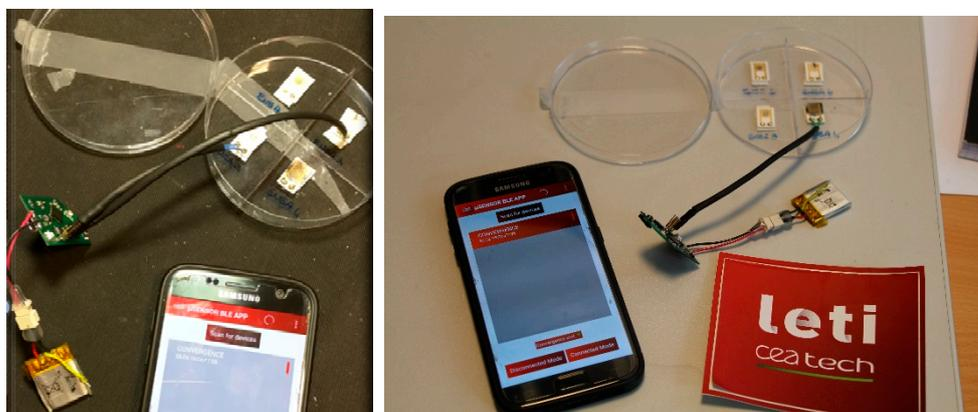
Figure 18. The graphene-based NO<sub>2</sub> sensors connected to the CEA-LETI platform.
