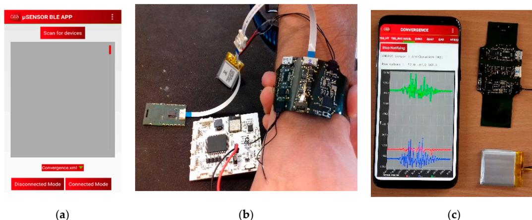
**Figure 9.** (a) Application interface (b) Flexible sensor platform tested with ISFET and activity sensor from EPFL and EDI—(c) Flexible sensor platform tested with embedded sensors.
