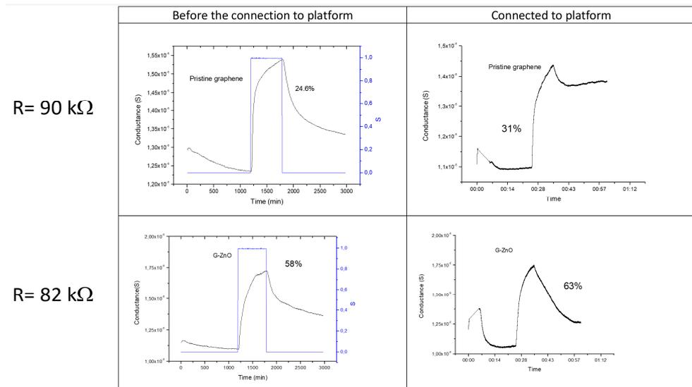
**Figure 20.** Sensing responses of the newly prepared devices, based on pristine and decorated graphene, exposed to 1 ppm of  $\text{NO}_2$  for 10 min. Figure is cut off.
