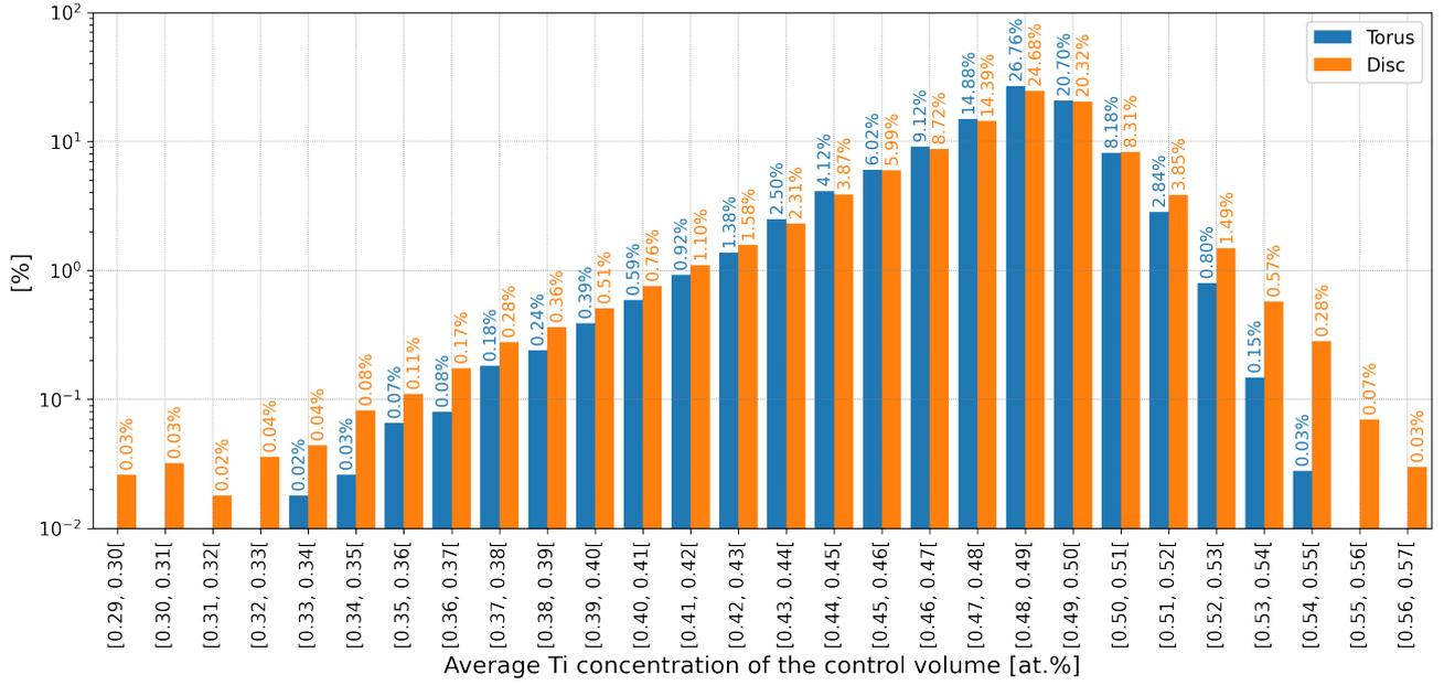
Figure 16: The density histograms of the average Ti concentration in the APT volume of Ni-Ti, given by the toroidal and disc-like RIS models.  $\bar{r}_1 = 7.0$  nm is the average loop radius. The nominal Ti concentration  $C_{\text{Ti}}^n$  is set to 0.48 at.%, the temperature is 450 °C, and the damage production rate is  $8 \times 10^{-5}$  dpa/s.
