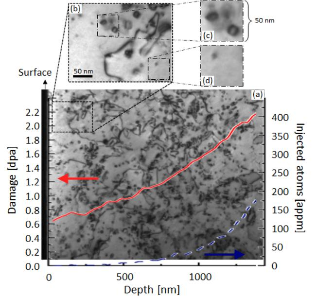
Figure 4: Microstructure of the irradiated Ni-Ti sample characterized by transmission electron microscopy. The solid and dashed lines respectively represent the irradiation damage and injected atom profiles given by SRIM.
