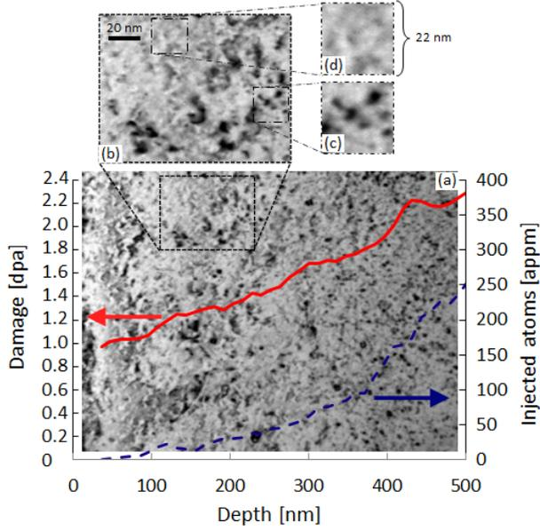
Figure 2: Microstructure of an irradiated Fe-Ni sample characterized by transmission electron microscopy. The solid and dashed lines respectively represent the irradiation damage and injected atom profiles calculated by the Stopping Range of Ions in Matter (SRIM) code [72] using the Kinchin-Pease option with a displacement threshold energy of 40 eV [73].
