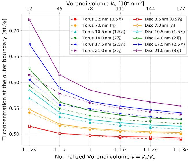
Figure 14: The distribution of the Ti concentration at the outer boundary in Ni-Ti obtained with different Voronoi volumes and dislocation loop radii, given by the toroidal and disc-like RIS models.  $\bar{r}_1 = 7.0$  nm is the average loop radius. The nominal Ti concentration  $C_{\text{Ti}}^{\text{N}}$  is set to 0.48 at.%, the temperature is 450 °C, and the damage production rate is  $8 \times 10^{-5}$  dpa/s.
