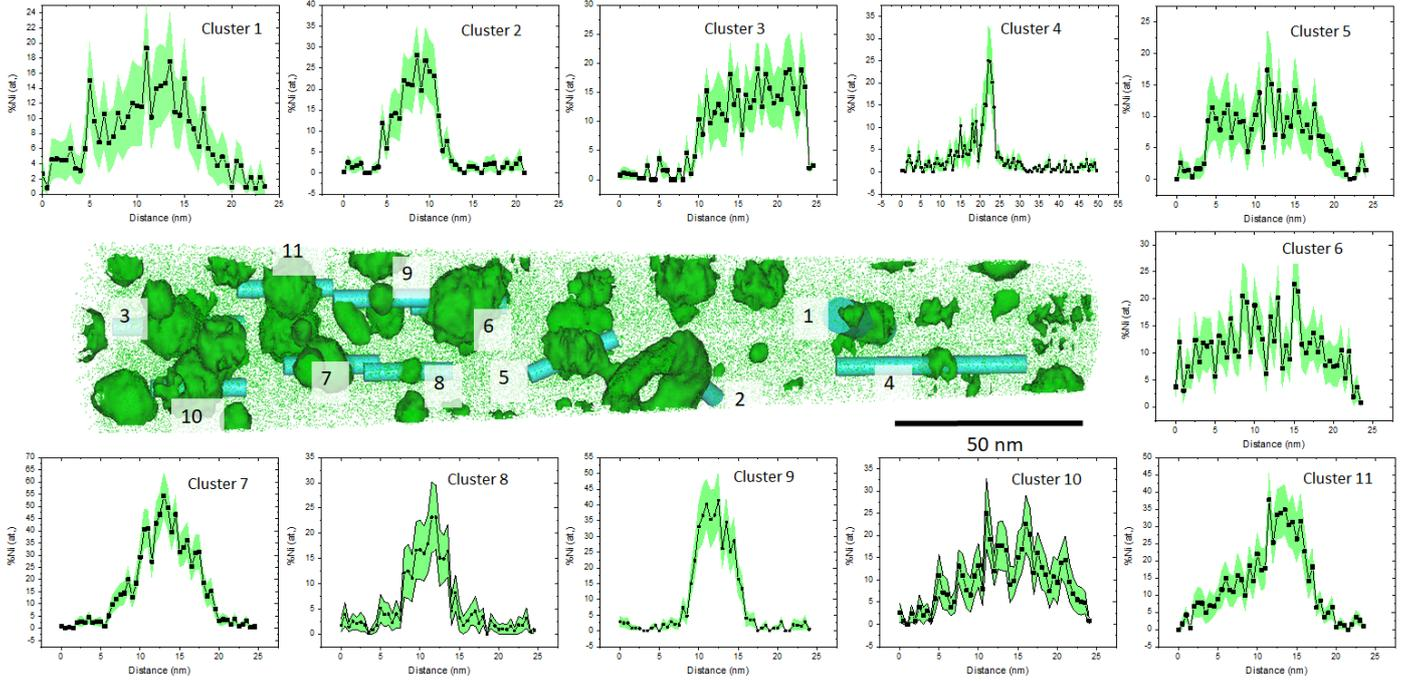
Figure 6: APT analysis of nickel (in green) distribution in Fe-Ni (in the middle) and the uni-dimensional depletion profiles crossing segments of potential dislocation loops. The square symbols of the uni-dimensional profiles represent the measured local Ni composition, and the shaded areas indicate the uncertainty domain.
