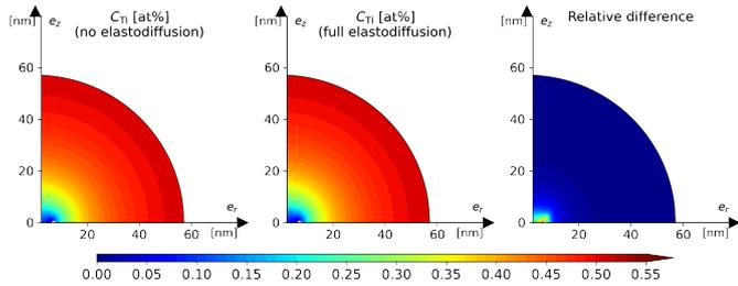
Figure 23: The Ti concentration fields around a dislocation loop in Ni-Ti obtained with and without considering the elastodiffusion; and the relative difference between these two concentration fields. The loop radius and the Voronoi’s volume are set to their average values, respectively. The effective nominal Ti concentration  $C_{\text{Ti}}^n$  is set to 0.48 at.%, the temperature is 450 °C, and the damage production rate is  $8 \times 10^{-5}$  dpa/s.
