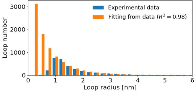
Figure 3: Histograms of the dislocation loop radius distribution in the irradiated Fe-Ni sample as measured by TEM, and interpolated by the gamma distribution function.
