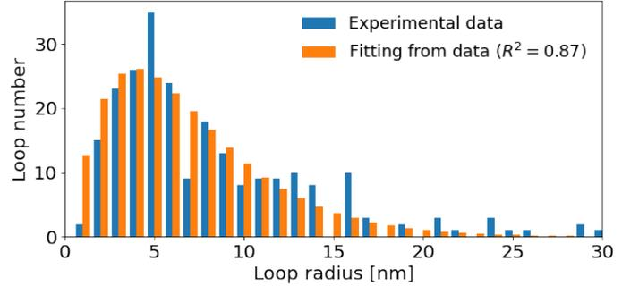
Figure 5: Histograms of loop radius in irradiated Ni-Ti obtained from experimental measurement and fitting from these data using the gamma distribution function.
