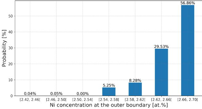
Figure 11: Calculated probabilities of the bulk Ni concentration at the outer boundary in Fe-Ni to be in the concentration intervals indicated by the x-axis. The effective nominal Ni concentration  $C_{\text{Ni}}^n$  is set to 2.70 at.%, the temperature is 400 °C, and the damage production rate is  $9 \times 10^{-4}$  dpa/s.
