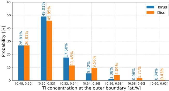
Figure 15: The probabilities for the Ti concentration at the outer boundary in Ni-Ti to be in different value ranges, given by the toroidal and disc-like RIS models.  $\bar{r}_1 = 7.0$  nm is the average loop radius. The nominal Ti concentration  $C_{\text{Ti}}^{\text{N}}$  is set to 0.48 at.%, the temperature is 450 °C, and the damage production rate is  $8 \times 10^{-5}$  dpa/s.
