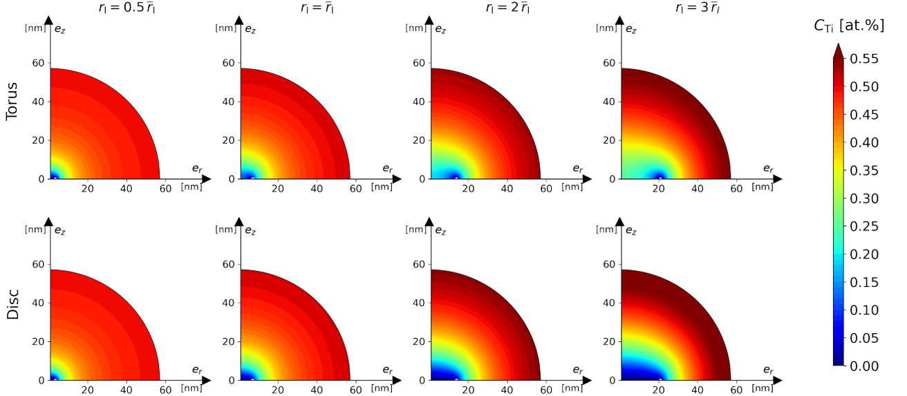
Figure 13: The Ti concentration field around a dislocation loop in Ni-Ti with toroidal (up) and disc-like (down) RIS regions for various loop radii.  $\bar{r}_l = 7.0 \text{ nm}$  is the average loop radius. The Voronoi's volume is set to its average value ( $7.7 \times 10^5 \text{ nm}^3$ ). The effective nominal Ti concentration  $C_{\text{Ti}}^n$  is set to 0.48 at.%, the temperature is 450 °C, and the damage production rate is  $8 \times 10^{-5} \text{ dpa/s}$ .
