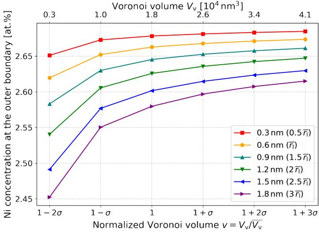
Figure 10: The distribution of the bulk Ni concentration at the outer boundary in Fe-Ni obtained for various Voronoi's volumes and dislocation loop radii.  $\bar{r}_1 = 0.6$  nm is the average loop radius. The effective nominal Ni concentration  $C_{\text{Ni}}^n$  is set to 2.70 at.%, the temperature is 400 °C, and the damage production rate is  $9 \times 10^{-4}$  dpa/s.
