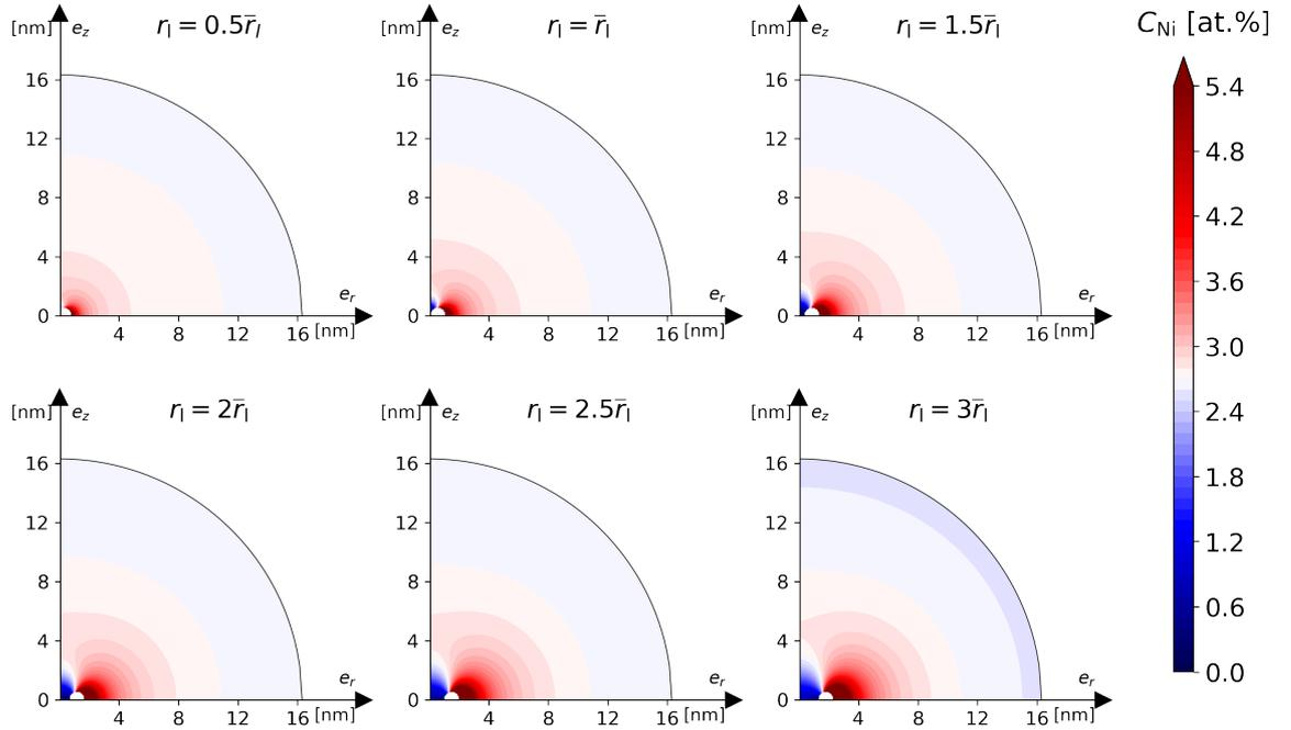
Figure 9: The Ni concentration distribution around a dislocation loop for in Fe-Ni various loop radii.  $\bar{r}_l = 0.6 \text{ nm}$  is the average loop radius. The Voronoi's volume is set to its average value ( $1.8 \times 10^4 \text{ nm}^3$ ). The effective nominal Ni concentration  $C_{\text{Ni}}^n$  is set to 2.70 at.%, the temperature is 400 °C, and the damage production rate is  $9 \times 10^{-4} \text{ dpa/s}$ .
