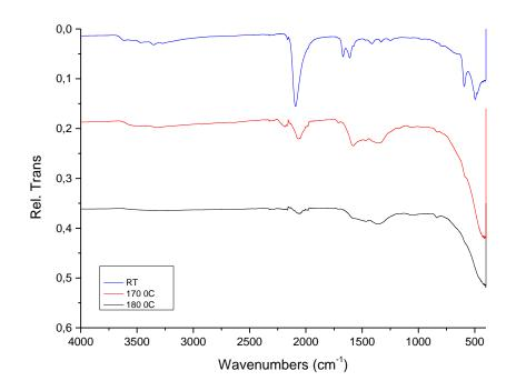
Figure 9: FT-IR of batch 4 at room T (blue) and after heating at 170  $^{\circ}$ C (red) and 180 $^{\circ}$ C (black). the v(CN) stretch has decreased in strength by 75 %.
