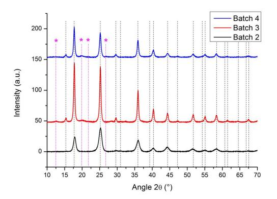
Figure 2: XRD of batches 2 (black), 3 (red) and 4 (green). The black dotted vertical lines are the Bragg reflections for a Fm3m space group. The purple vertical lines indicated with an asterisk are respectively the 1<sup>st</sup>, 4<sup>th</sup>, 5<sup>th</sup> and 7<sup>th</sup> supplementary Bragg reflections from a Pm3m space group (remaining reflections were either superimposed with the Fm3m ones or omitted for clarity)
