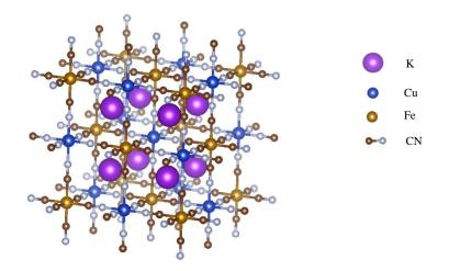
Figure 1: Schematic representation of the structure of K<sub>2</sub>CuFe(CN)<sub>6</sub> in which none of the Fe sites are vacant.
