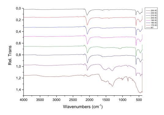
Figure 7: FT-IR of batch 2 at room temperature, as well as after various heat treatments from 170 0C to 250 0C. Each scan corresponds to 4 hours at that temperature. The sample is the same one throughout the experiment.
