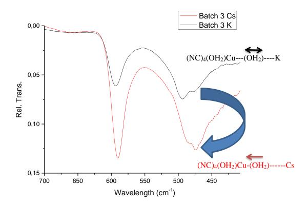
Figure 11: FT-IR of batch 3 before (black) and after (red) Cs/K exchange. Note the inversion of the relative strength of the v(Cu-N) stretches.
