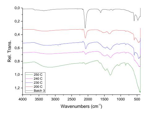
Figure 10: FT-IR of Cs exchanged batch 3 taken before thermal treatment began (black) and after thermal treatment at 200, 230, 240 and  $250^{\circ}$ C.
