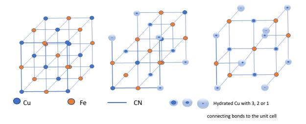
Figure 5: From left to right Cu-HCF with 0, 20, and 50 % of the  $Fe(CN)_6^{4-}$  sites vacant. As the number of vacancies increase the materials dependence on water to complete the structure increases.
