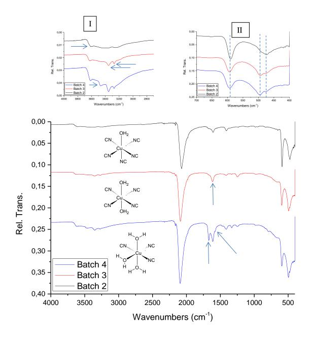
Figure 3: FT-IR of batches 2 (black), 3 (red) and 4 (blue) Cu-HCF. Note the increase in the number of co-ordinated water peaks as the copper to iron ratio is increased.
