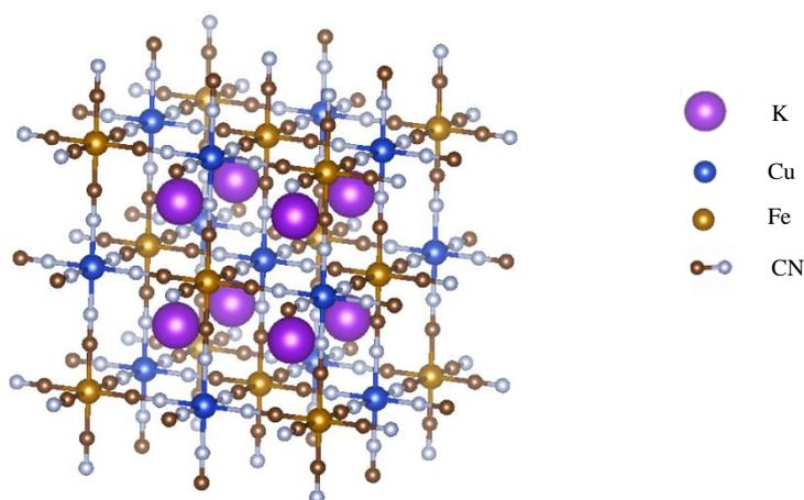
Figure 1: Schematic representation of the structure of K<sub>2</sub>CuFe(CN)<sub>6</sub> in which none of the Fe sites are vacant.
