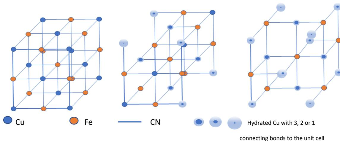
Figure 5: From left to right Cu-HCF with 0, 20, and 50 % of the Fe(CN)<sub>6</sub><sup>4-</sup> sites vacant. As the number of vacancies increase the materials dependence on water to complete the structure increases.
