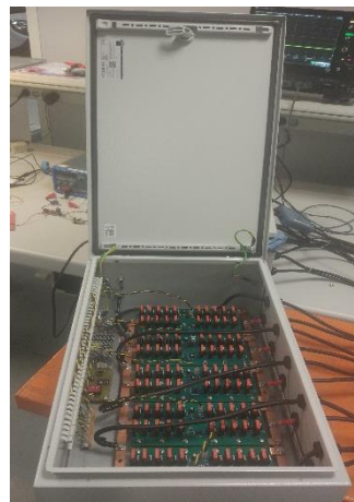
Figure 4: Photography of a wired 10 kA switch under test
