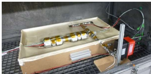
Fig 2 - Closed vessel equipped with pressure and thermal sensors
