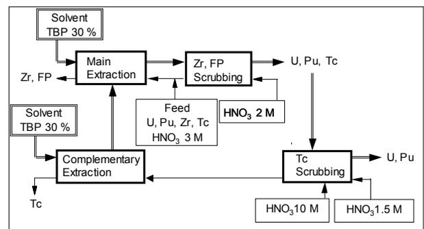
Figure 2. Flow-sheet of the 1<sup>st</sup> PUREX extraction cycle employed at Cogema La Hague.
