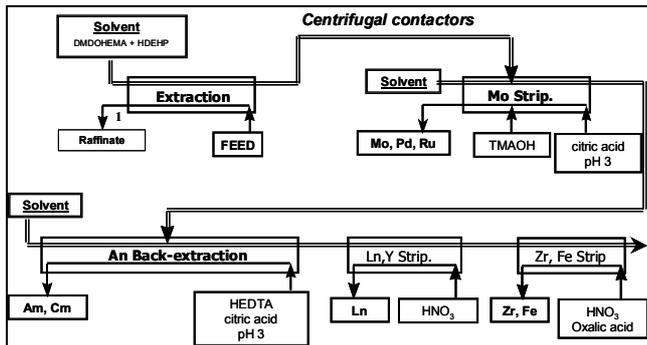
Figure 3. Flowsheet of the DIAMEX-SANEX process tested on genuine solution in 2000.
