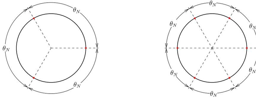
**Figure 5.**  $N$  pairs of transducers evenly arranged around the pipe, every  $\theta_N = 2\pi/N$  ( $N \geq 2$ ), to get rid of the bending effects by summation of their mechanical strains variation measurement – Examples for  $N = 3$  (left) and  $N = 6$  (right).
