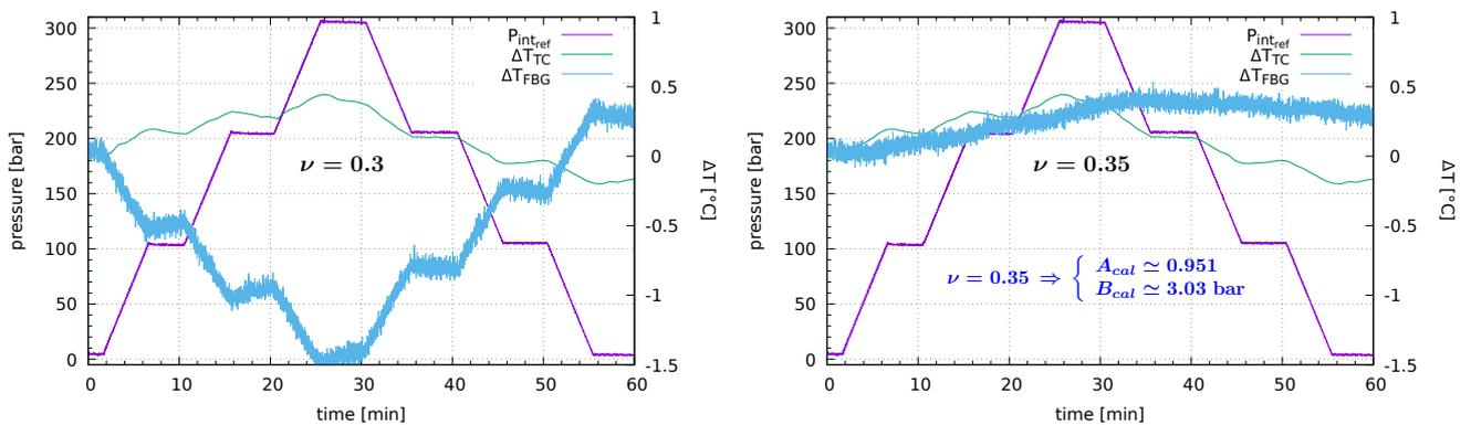
**Figure 8.** Results of the pressure test held at Technip Energies facility in Marseille in July 2019 – With additional surface temperature variation computed from FBG measurements ( $\nu = 0.3$  (left) &  $\nu = 0.35$  (right)).
