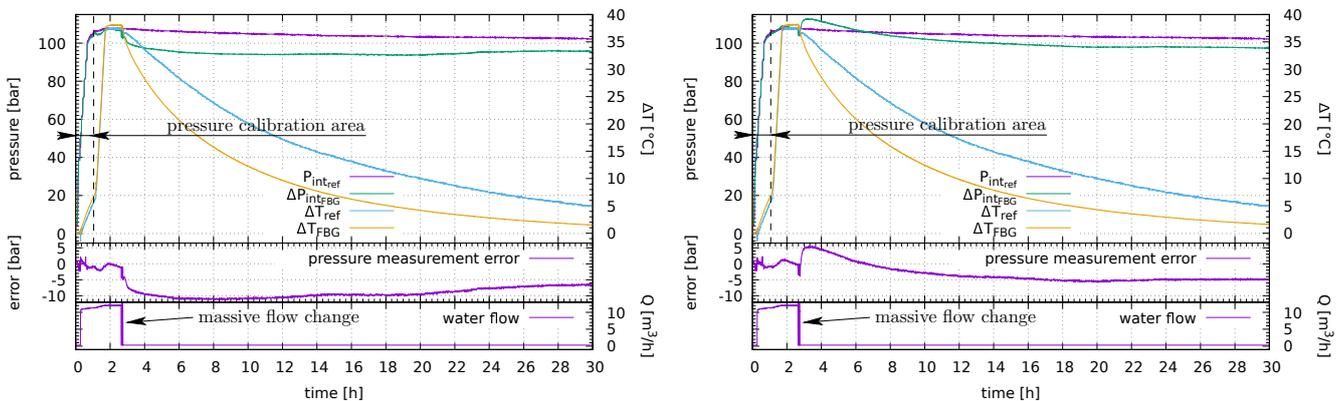
**Figure 14.** Last pressure test with fluid flow & temperature changes ( $\varnothing$  2" NPS Sch. 80) – Single sensor (left) vs. two sensors average measurements to mitigate potential bending effects resulting from massive flow change (right).
