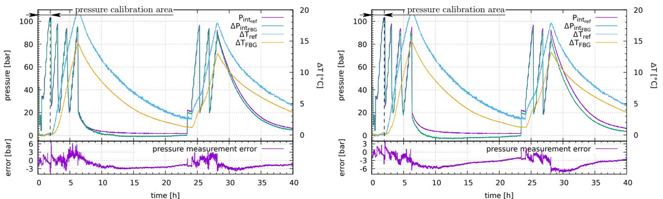
**Figure 13.** Second pressure test with no fluid flow & temperature changes ( $\varnothing$  4" NPS Sch. 160) – Single sensor (left) vs. three sensors average measurements to mitigate potential bending effects (right).
