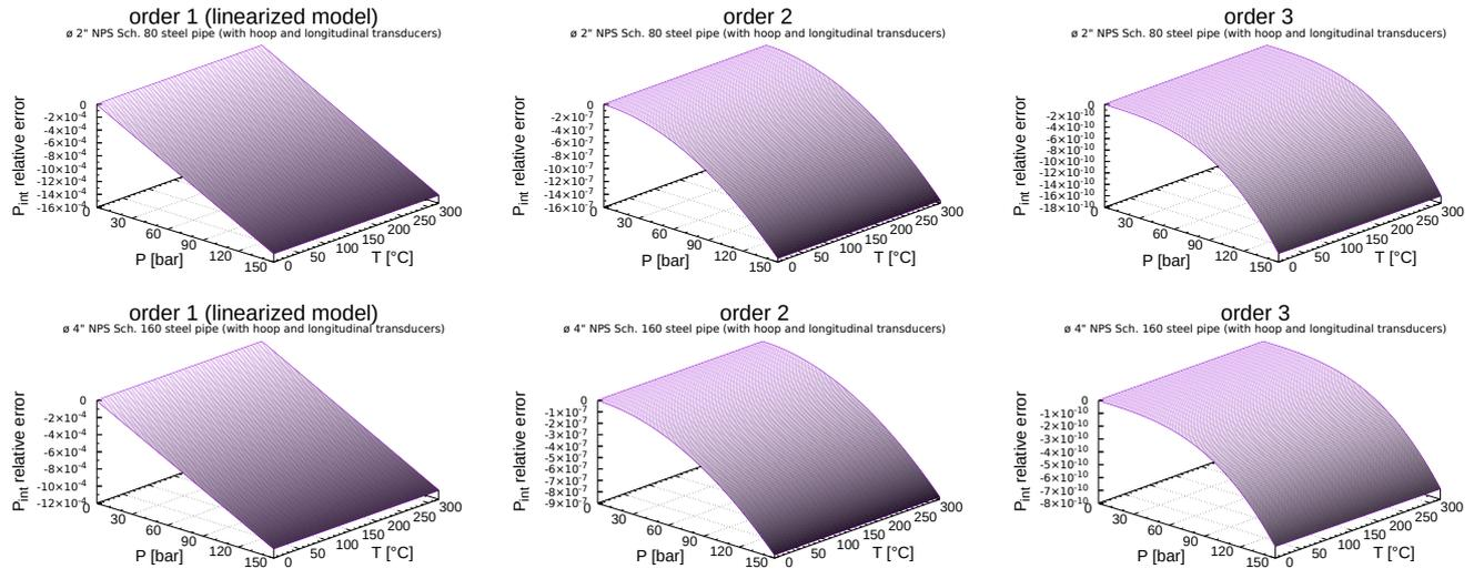
**Figure 2.** Iterative model relative error for  $P_{int}$ , from initialization (linear approximation – order 1) to iteration 2 (order 3) ( $P_{ref} = 0$  bar &  $T_{ref} = 0$  °C) – First row:  $\varnothing$  2" NPS Sch. 80 steel pipe – Second row:  $\varnothing$  4" NPS Sch. 160 steel pipe.
