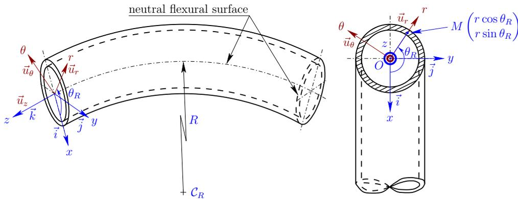
**Figure 4.** Bended pipe – Relationship between the local cartesian coordinate system  $(O, x, y, z)$  used to describe the bending model, and the cylindrical coordinate system  $(O, r, \theta, z)$  used so far to establish the formal model for the infinitely long and straight pipe under hydrostatic pressure.
