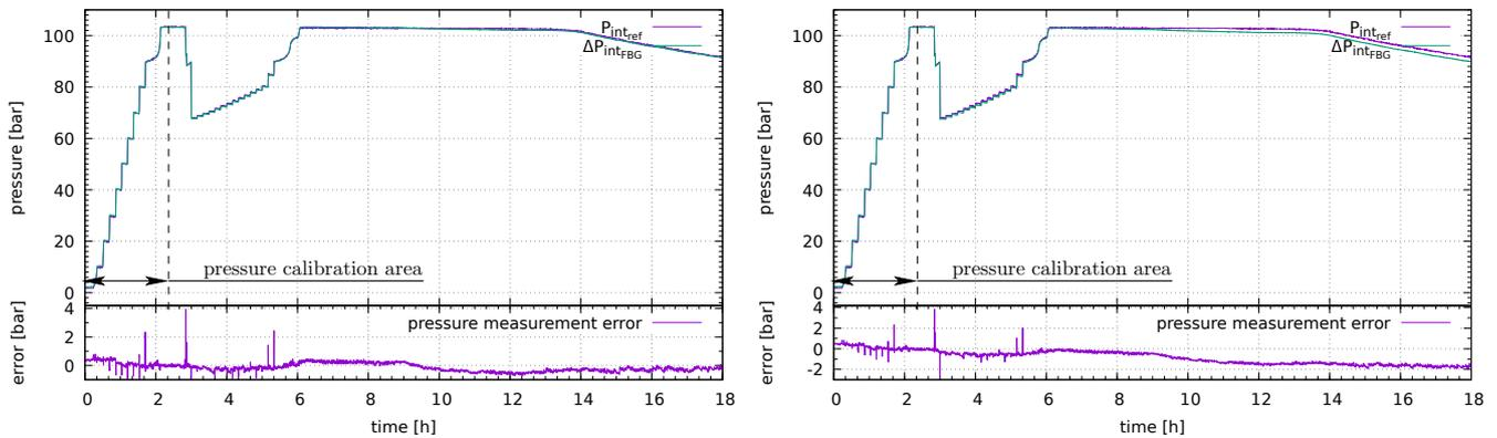
**Figure 12.** First pressure test with no fluid flow & fluid constant temperature ( $\varnothing$  4" NPS Sch. 160) – Single sensor (left) vs. three sensors average measurements to mitigate potential bending effects (right).
