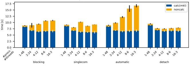
node scaling: per thread runtime (48 total threads)
