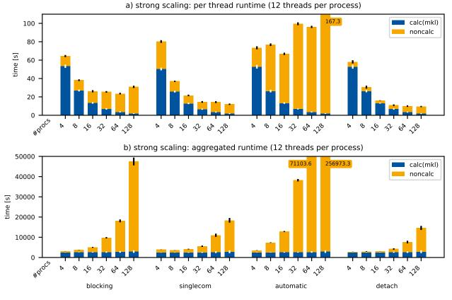
Figure 2: Strong scaling measurements of distributed Block Cholesky Factorization
