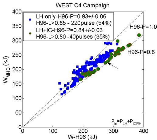
Figure 8. Stored energy of WEST discharges versus ITER-L-96P scaling law for LHCD only (squares) and LHCD+ICRH (circles) discharges.
