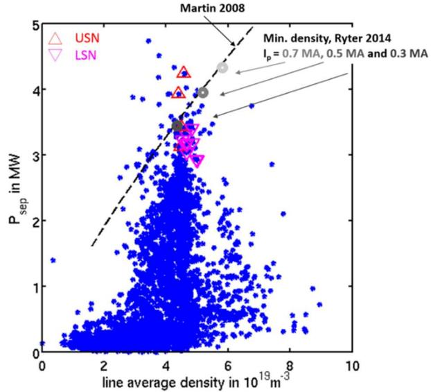
Figure 13.  $P_{sep}$  versus density for the whole C4 campaign. The dashed line is the Martin's scaling for L-H transition ( $B=3.7T$ ).
