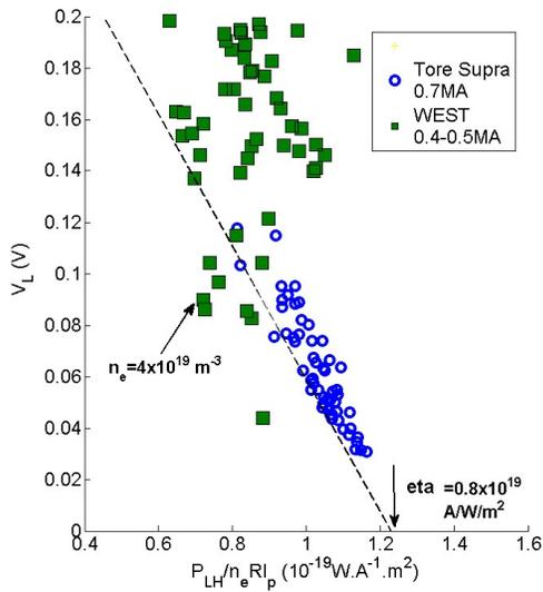
Figure 14. Loop voltage as a function of normalized LHCD power. All pulses below the dashed line with  $50mV < V_L < 110mV$  are in upper single-null configuration
