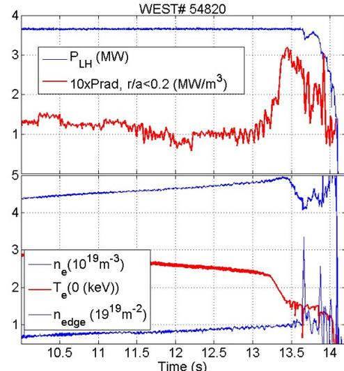
Figure 7. Thermal instability of a LHCD discharge
