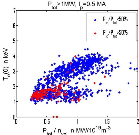
Figure 6. Central electron temperature for LHCD and ICRH dominated discharges
