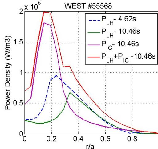
Figure 11. Power deposition of the discharge of figure 12 (METIS modeling)
