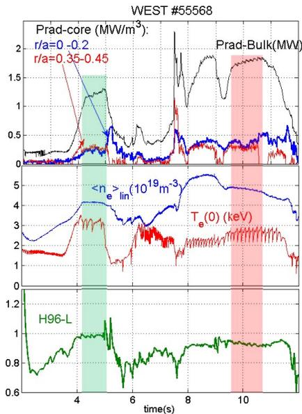
Figure 10. Discharge with a 3MW LHCD-only phase (green shaded) and a LHCD+ICRH phase (2MW+3MW, red shaded)
