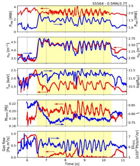
Figure 12. 4-second H-mode discharge in LSN configuration. Total power  $P_{tot}$  is the combination of 4MW of LHCD with 1MW of ICRH.
