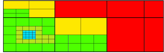
Fig. 3.5 A 2-dimensional AMR mesh obtained with 5 levels of successive binary refinements of 4 \times 2 rectilinearly aligned hypertree objects with different sizes along each axis. Here, different colors are used to represent the level of each cell, i.e. red for unrefined hypertrees and blue for the finest meshes.
