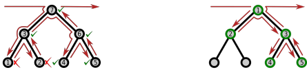
Fig. 5.6 Stages of a two-stage filter applied to one constituting hypertree within a binary hypertree grid. Left: pre-processing stage with post-order DFS traversal, using a lightweight cursor, selecting vertices check-marked in green. Right: main stage with pre-order DFS traversal with a heavier cursor, only across pre-selected vertices. The indices reflect the order in which vertices are processed by each stage.
