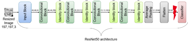
Figure 2: Pre-trained ResNet50 architecture Convolutional Block extracts features while changing the input dimension. Identity Block enables to extract features without changing input dimension.
