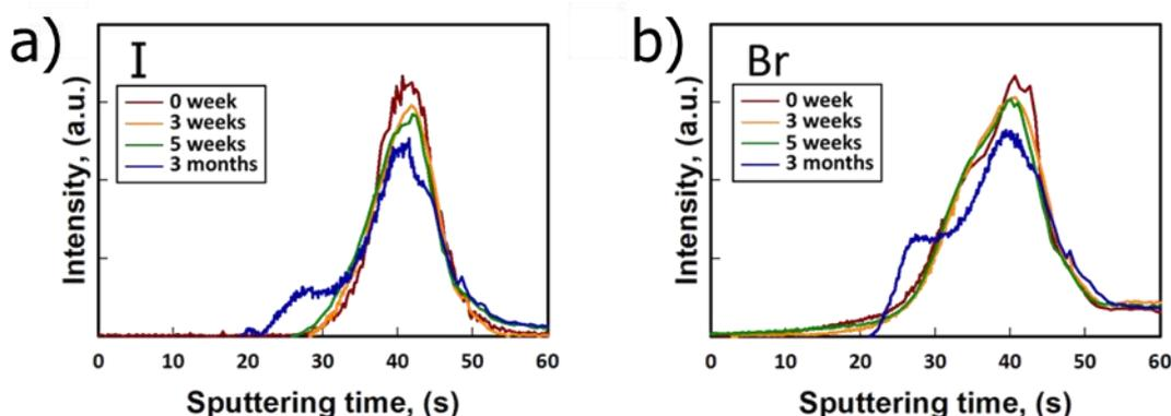
Figure 1. GD-OES profile lines showing a) iodide and b) bromide ion diffusion toward silver top electrode.
