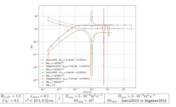
Figure 16: Evolution of We dimensionless number when varying  $r^0$ ,  $Sh_{met}$  and  $D_{met} - (\rho_{met,eq} > \rho_{oxy,eq})$
