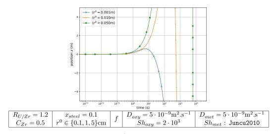
Figure 14: Evolution of position z when varying  $r^0 - (\rho_{met,eq} > \rho_{oxy,eq})$  - the y-axis range has been truncated
