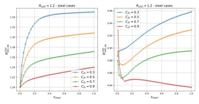
Figure 5:  $R_{oxy}^{U/Zr}$ ,  $R_{met}^{U/Zr}$  at equilibrium for  $R_{U/Zr} = 1.2$ ,  $C_{Zr} \in [0.3, 0.9]$ ,  $x_{steel} \in [5 \cdot 10^{-3}, 1]$  - steel = {68.67% Fe, 20.72% Cr, 10.61% Ni} case
