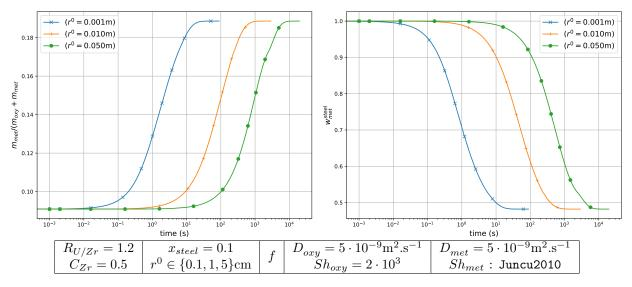
Figure 11: Evolution of the metal phase relative mass and  $w_{met}^{steel}$  when varying  $r^0 - (\rho_{met,eq} > \rho_{oxy,eq})$
