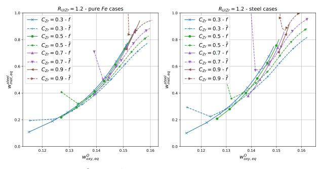
Figure 6: f and  $\tilde{f}$  functions  $w_{oxy,eq}^O \mapsto w_{met,eq}^{steel}$  for  $R_{U/Zr} = 1.2$  and  $C_{Zr} \in \{0.3, 0.5, 0.7, 0.9\}$
