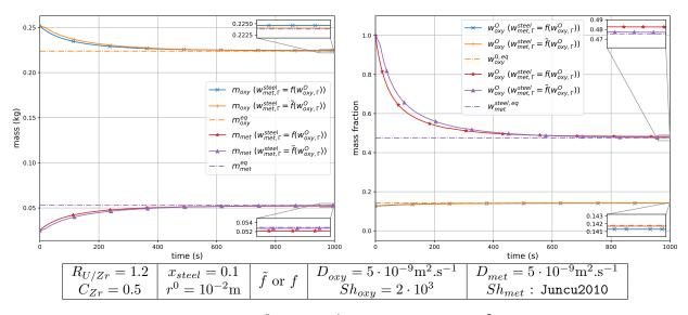
Figure 7: Evolution of  $m_{oxy}$ ,  $m_{met}$ ,  $w_{oxy}^O$  and  $w_{met}^{steel}$  towards equilibrium with  $\tilde{f}$  or  $f - (\rho_{met,eq} > \rho_{oxy,eq})$
