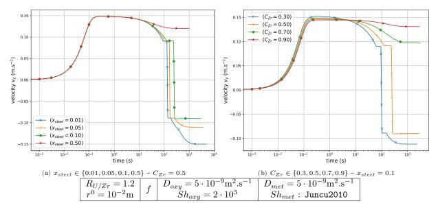
Figure 18: Evolution of velocity  $v_z$  when varying  $x_{steel}$  or  $C_{Zr}$
