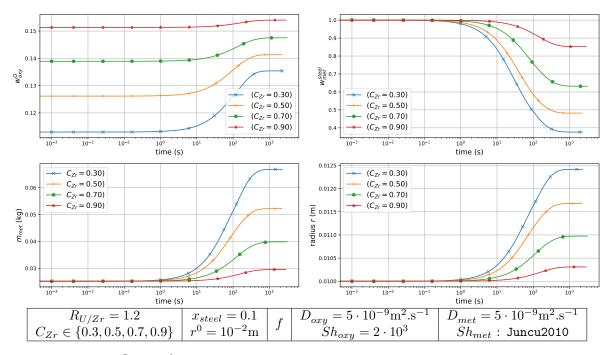
Figure 10: Evolution of  $w_{oxy}^O$ ,  $w_{met}^{steel}$ ,  $m_{met}$  and the droplet radius when varying  $C_{Zr} - (\rho_{met,eq} > \rho_{oxy,eq})$  for  $C_{Zr} \in \{0.3, 0.5\}$ ,  $(\rho_{met,eq} < \rho_{oxy,eq})$  for  $C_{Zr} \in \{0.7, 0.9\}$
