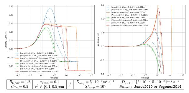
Figure 15: Evolution of velocity  $v_z$  and position z when varying  $r^0$ ,  $Sh_{met}$  and  $D_{met} - (\rho_{met,eq} > \rho_{oxy,eq})$  - the y-axis range has been truncated for the position
