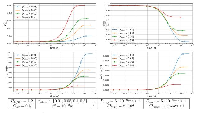
Figure 9: Evolution of  $w_{oxy}^O$ ,  $w_{met}^{steel}$ ,  $m_{met}$  and the droplet radius when varying  $x_{steel} - (\rho_{met,eq} > \rho_{oxy,eq})$  for  $x_{steel} \in \{0.01, 0.05, 0.1\}$ ,  $(\rho_{met,eq} < \rho_{oxy,eq})$  for  $x_{steel} \in \{0.5\}$
