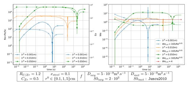
Figure 13: Evolution of  $Re_{met} = Pe_{met}/Sc$ , Eo and We dimensionless numbers when varying  $r^0 - (\rho_{met,eq} > \rho_{oxy,eq})$
