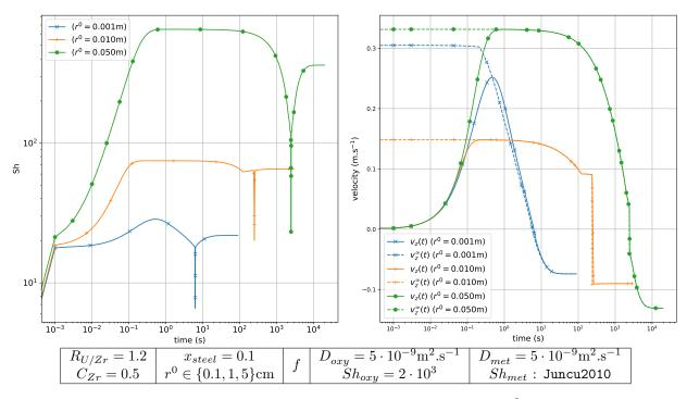
Figure 12: Evolution of  $Sh_{met}$ , dimensionless number and velocity  $v_z$  when varying  $r^0 - (\rho_{met,eq} > \rho_{oxy,eq})$
