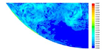
Figure 17: Computational Fluid Dynamics simulation of a BALI [31] experimental configuration using "Large Eddy Simulation" for turbulence - velocity modulus  $(m.s^{-1})$  – extracted from [32]
