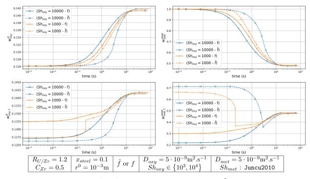
Figure 8: Evolution of  $w_{met}^{steel}$ ,  $w_{oxy}^O$ ,  $w_{oxy,\Gamma}^O$  and  $w_{met,\Gamma}^{steel}$  when varying  $Sh_{oxy}$  with  $\tilde{f}$  or  $f - (\rho_{met,eq} > \rho_{oxy,eq})$
