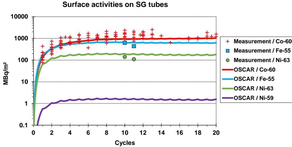
Figure 8. OSCAR V1.4 calculation/Measurements comparison for  $^{60}\text{Co}$ ,  $^{55}\text{Fe}$  and  $^{63}\text{Ni}$  surface activities on SG tubes.
