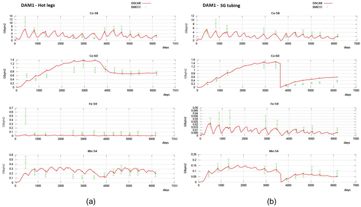
Figure 6. DAMPIERRE-1 – OSCAR V1.4 calculation/EMECC measurements comparison for <sup>58</sup>Co, <sup>60</sup>Co, <sup>59</sup>Fe and <sup>54</sup>Mn activities deposited on the hot legs (a) and the SG tubing (b).
