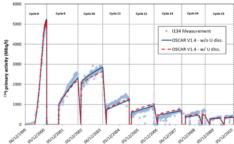
Figure 7. CATTENOM-3 – OSCAR V1.4 calculation/Measurement comparison for <sup>134</sup>I primary activity during power operating cycles.
