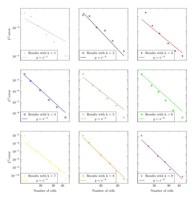
Figure 8:  $L^2$ -error with symmetric scheme and random mesh for problem of Sec. 4.2.
