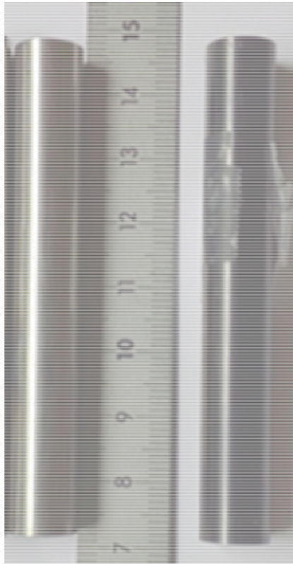
Photo of Zy4 claddings. Some Zy4 claddings were artificially oxidized.
