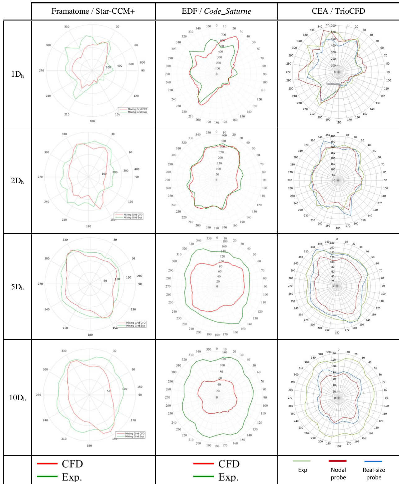
242 Figure 9. Polar representation of pressure standard deviation distribution around the central rod 243 (red curves for CFD velocities, green curves for experimental velocities, blue curves do not have to 244 be considered for this comparison)
