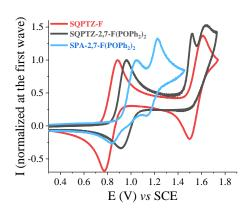
Figure 1. Cyclic voltammetry in reduction (Left, DMF + Bu<sub>4</sub>NPF<sub>6</sub> 0.1 M, sweep-rate 100 mV.s<sup>-1</sup>) and in oxidation (Right, CH<sub>2</sub>Cl<sub>2</sub> + Bu<sub>4</sub>NPF<sub>6</sub> 0.2 M, sweep-rate 100 mV.s<sup>-1</sup>) of **SQPTZ-2,7-F(POPh<sub>2</sub>)<sub>2</sub>**, **SQPTZ-F** and **SPA-2,7-F(POPh<sub>2</sub>)<sub>2</sub>**.
