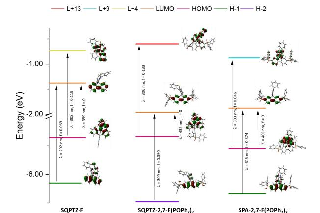
Figure 2. Representation of the energy levels and the main molecular orbitals involved in the electronic transitions of **SQPTZ-F**, **SQPTZ-2,7-F(POPh<sub>2</sub>)<sub>2</sub>** and **SPA-2,7-F(POPh<sub>2</sub>)<sub>2</sub>** obtained by TD-DFT b3lyp and the 6-311+G(d, p) basis set on the geometry of  $S_0$ , shown with an isovalues of 0.04 [e bohr- $^3$ ]<sup>1/2</sup> (for clarity purpose, only the main contribution for each transition is shown, details provided in SI).
