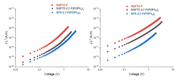
Figure 6. Thickness-scaled current voltage characteristics of  $SQPTZ-2,7-F(POPh_2)_2$  (black lines), SQPTZ-F (red lines) and  $SPA-2,7-F(POPh_2)_2$  (blue lines) hole-(Left) and
