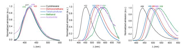
Figure 4. Emission spectra in different solvents of SQPTZ-F (Left), SQPTZ-2,7-F(POPh<sub>2</sub>)<sub>2</sub> (middle) and SPA-2,7-F(POPh<sub>2</sub>)<sub>2</sub> (Right).
