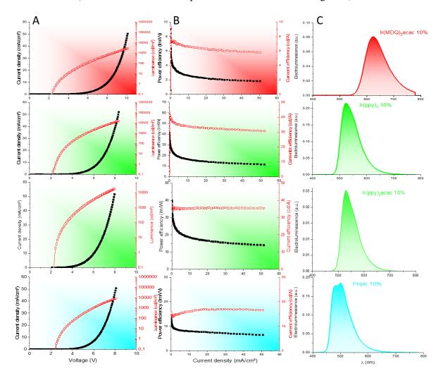
Figure 7. SL-PhOLEDs characteristics using  $SQPTZ-2,7-F(POPh_2)_2$  as host material. A) Current density (mA/cm²) and luminance (cd/m²) as a function of the voltage; B) Current efficiency (cd/A, filled symbols) and power efficiency (lm/W, empty symbol) as a function of the current density (mA/cm²) and C) Normalized EL spectra.
