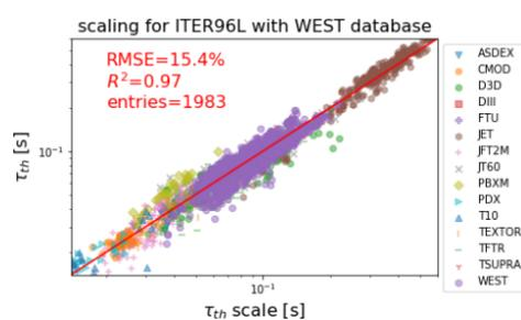
The aspect ratio does not play an important role in the scaling. Even if WEST has an aspect ratio larger than the other tokamaks in ITER96L database, the regression coefficient still close to zero.
