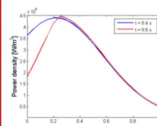
The increase of the tungsten in the center of the plasma is not sufficient to reproduce the collapse. The central value of the LHCD power deposition is reduced in an ad-hoc manner.
