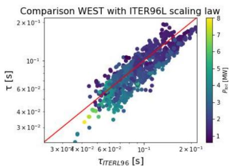
A weaker dependence on density is found. But WEST confinement time is well aligned with ITER96-L
