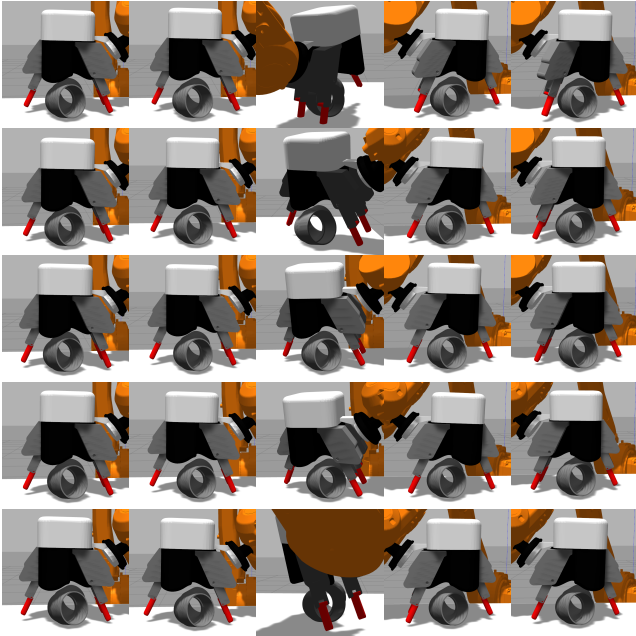
Fig. 5. Gripper configurations generated when visiting a two dimensional latent space. The central image is the point (0, 0) in latent space. The inner and outer image rings around it correspond to points evenly distributed on circles of diameter respectively 0.5 and 1 in latent space. Here, translations along the image plan normal are not visible, which explains some visually almost identical configurations.
